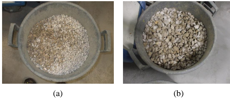
Fig. 4 – Crushed stone used in the test of the evaluation of injection of the grout by gravity: (a) Crushed stone 1 (6-12mm); (b) Crushed stone 2 (12-20mm)
