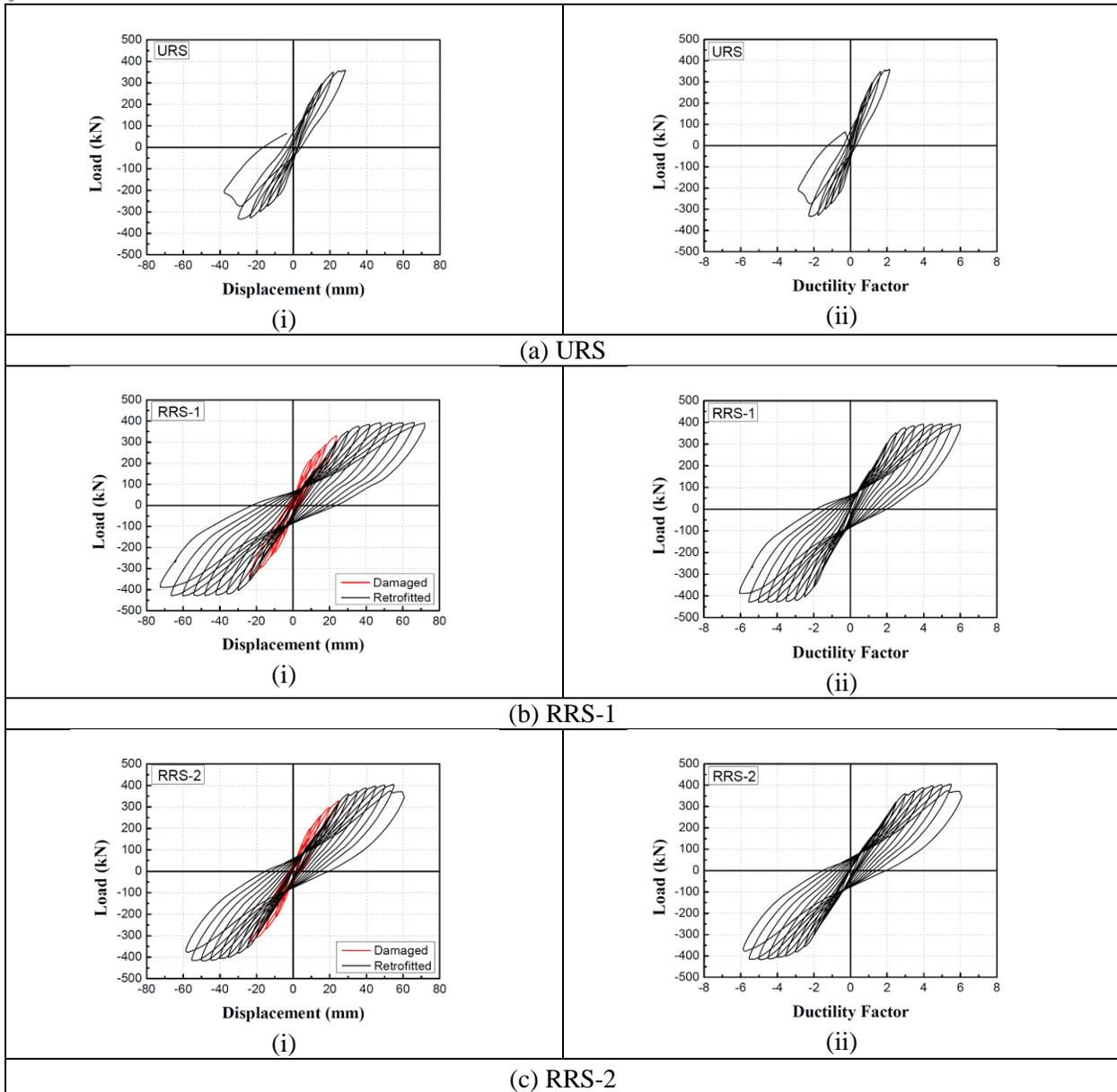
Fig. 4 – Experimental behavior of specimens ((i): Load-displacement, (ii): Load-ductility factor)
