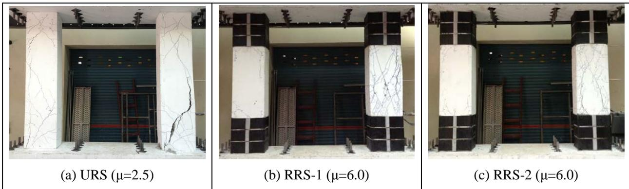
Fig. 6 – Final crack distribution
