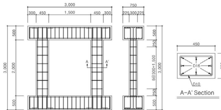
Fig. 2 – Detail of RC specimen (Unit=mm)
