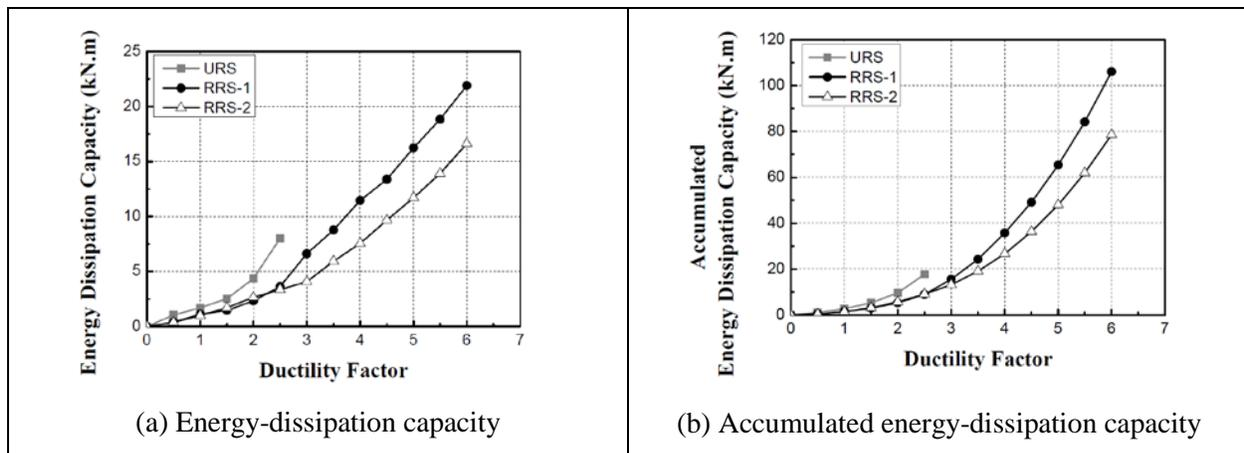
Fig. 7 – Hysteretic energy-dissipation capacity
