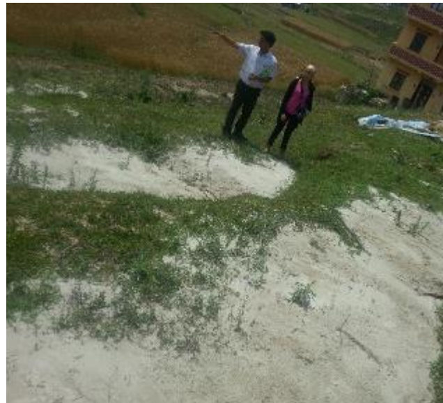
Fig. 8 – (a) Sand boils in Duwakot, Bhaktapur (b) Sand boils observed in the potato field with the fissures in Mulpani.
