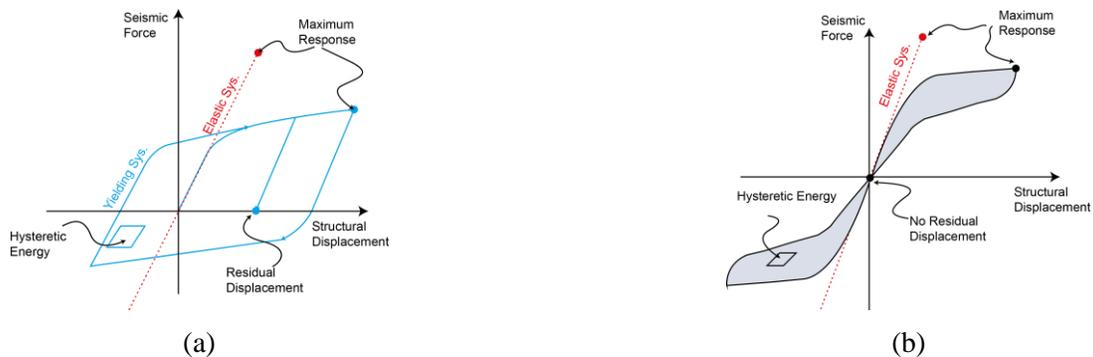
Fig. 1 - Idealized Force-Displacement Relationship: (a) Conventional Hysteresis; (b) SC System Hysteresis
