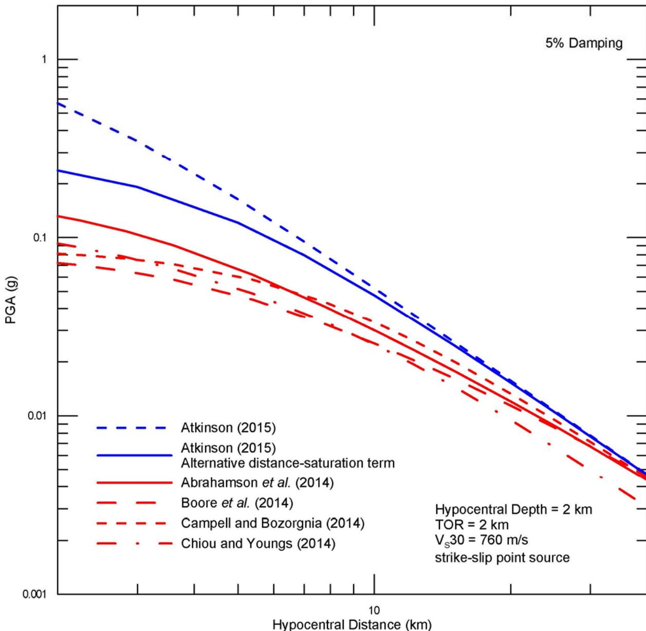
Fig. 3 – Ground motion prediction models for  $M$  4.5 used for induced earthquakes in U.S.
