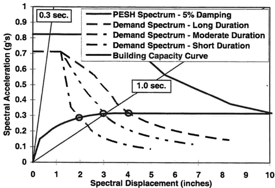
Fig. 6 – Example demand spectra – moderate-code building (M 7.0 at 20 km, western U.S., site class E). (Source: NIBS [12]).
