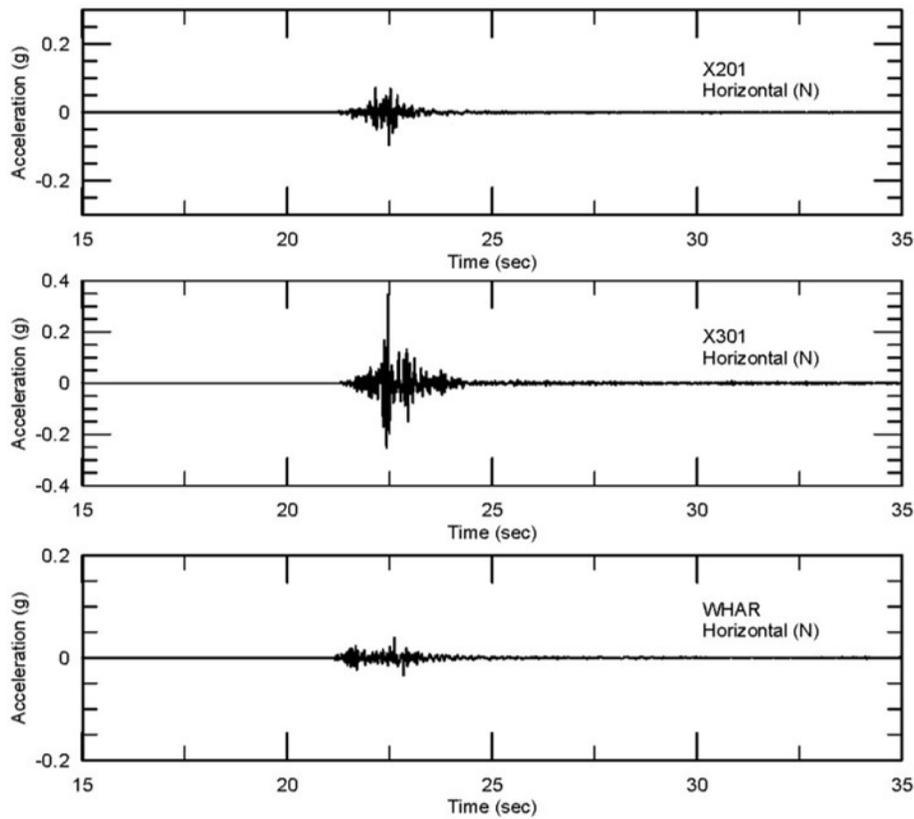
Fig. 5 – Acceleration time history of the 2013 M 4.1 Timpson, Texas earthquakes.
