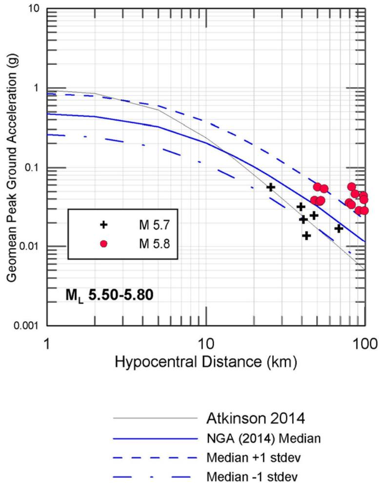
Fig. 4 – Comparison of PGA values from induced earthquakes in Oklahoma and Kansas with ground motion prediction models. The data shown in the last magnitude bin are for the 2011 Prague and 2016 Pawnee earthquakes. The site conditions are not known for the Oklahoma and Kansas seismic stations and so a  $V_{s30}$  of 370 m/sec has been assumed.
