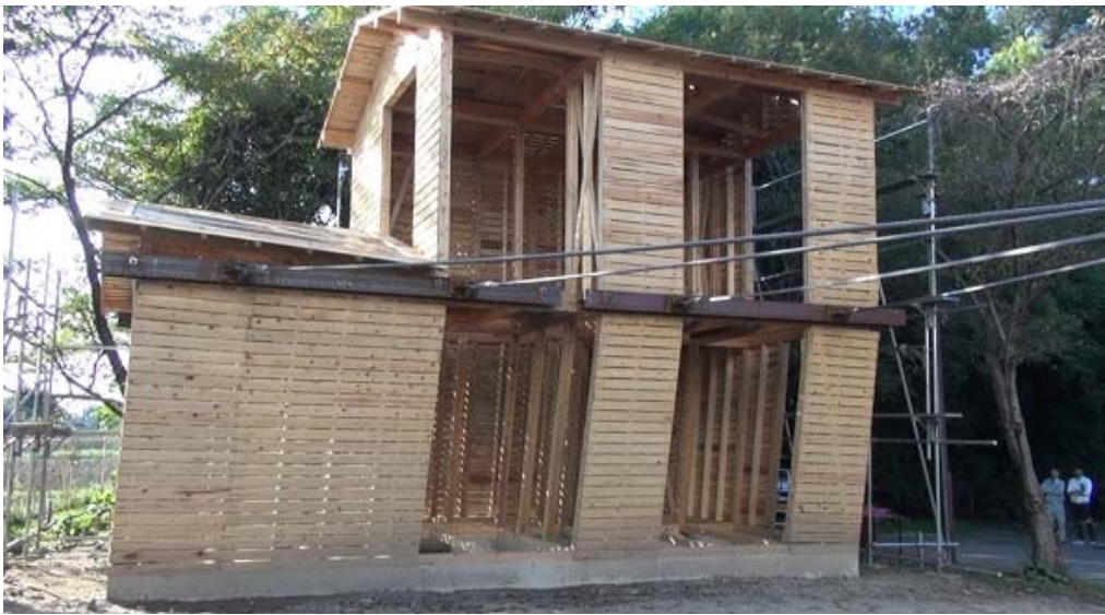
Photo 1 The final stage of the pull-down test just before the collapse in the case of “Without WoC”.
