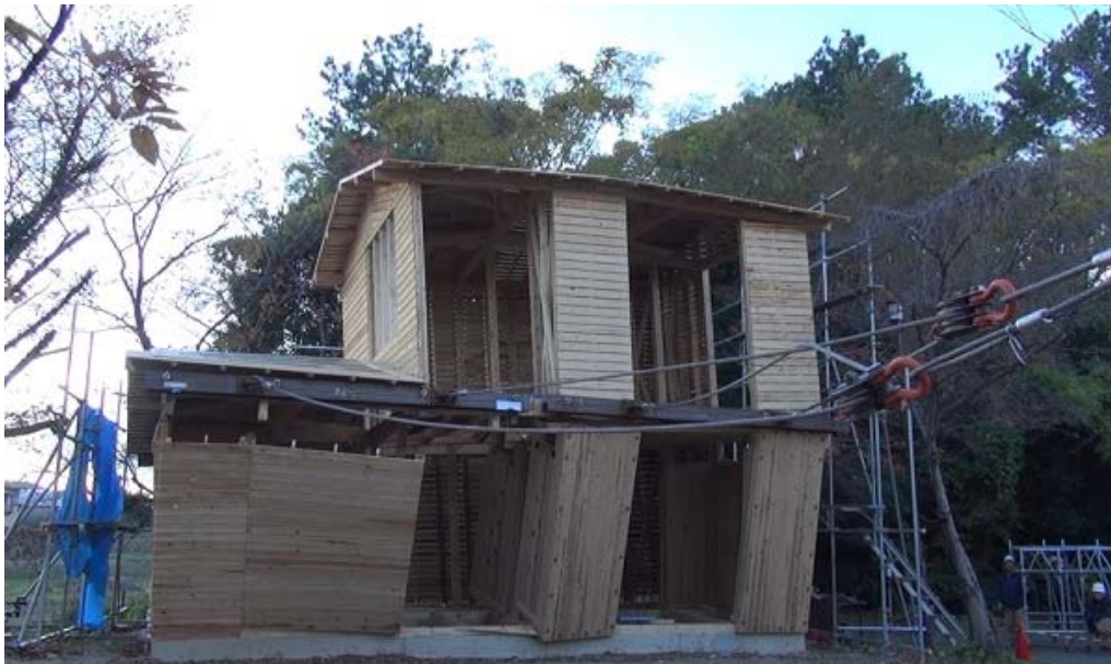
Photo 2 The final stage of the pull-down test just before the collapse in the case of “With WoC”.
