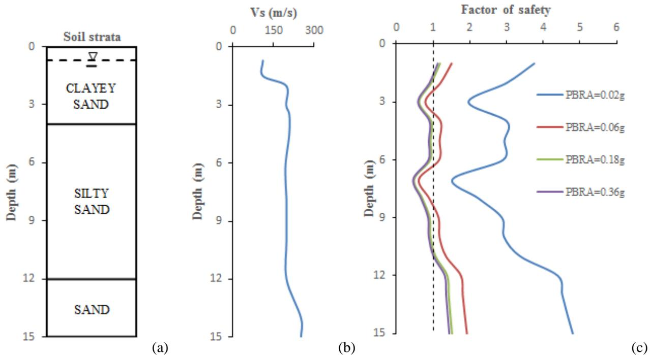
Fig. 13 - (a) Sub-surface soil profile at site BH3 (b) Shear wave velocity profile at site BH3 (c) FOS vs Depth for the four input motion components
