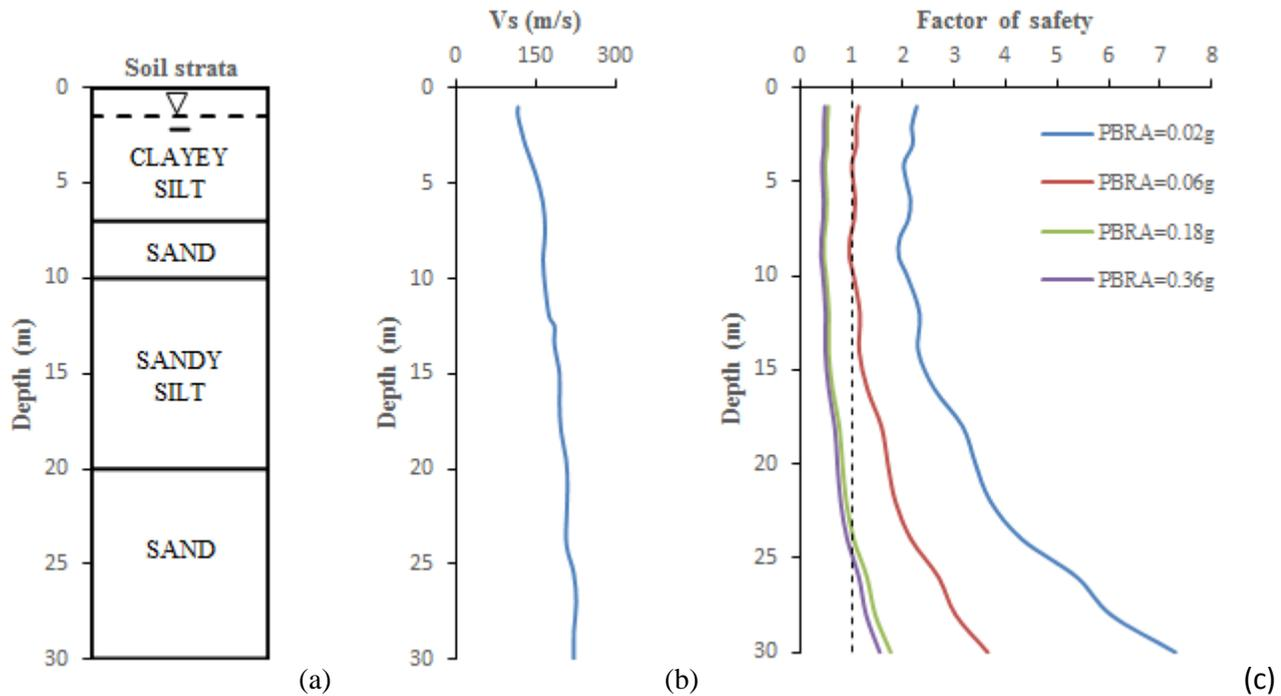
Fig. 10 - (a) Sub-surface soil profile at site BH2 (b) Shear wave velocity profile at site BH2 (c) FOS vs Depth for the four input motion components
