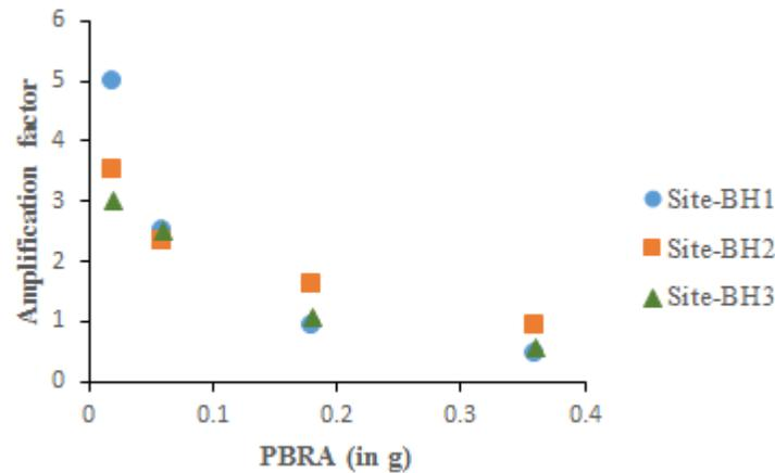
Fig. 14 - Effect of varying input motion PBRA on the amplification factor estimated for the three sites
