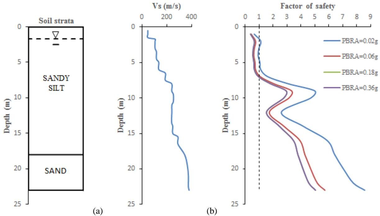
Fig. 7 – (a) Sub-surface soil profile at site BH1 (b) Shear wave velocity profile at site BH1 (c) FOS vs Depth for the four input motion components
