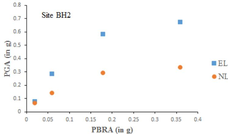
Fig. - 17 Effect of varying input motion PBRA on the PGA estimated from EL and NL approaches for site BH2
