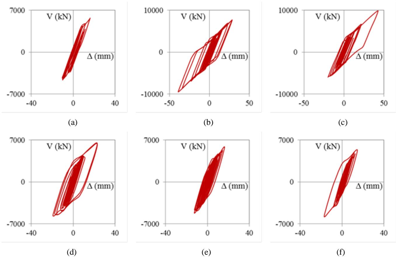
Fig. 8 – Hysteretic response of building III in orthogonal directions (a) displacement in the X direction for event 1, (b) displacement in the X direction for event 2, (c) displacement in the X direction for event 3, (d) displacement in the X direction for event 1, (e) displacement in the X direction for event 2, (f) displacement in the X direction for event 3
