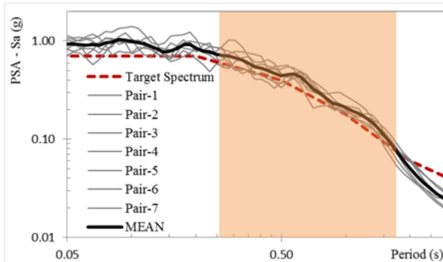
Fig. 2 – SRSS of the pseudo acceleration response spectrum (PSA) of the scaled records versus the target uniform hazard spectrum (UHS) for Building I
