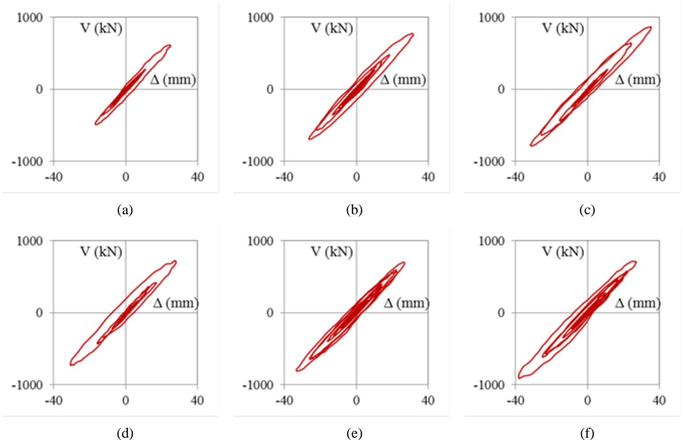
Fig. 3 – Hysteretic response of building I in the X direction subjected to six of the seismic events: (a) event 1, (b) event 2, (c) event 3, (d) event 4, (e) event 5, (f) event 6
