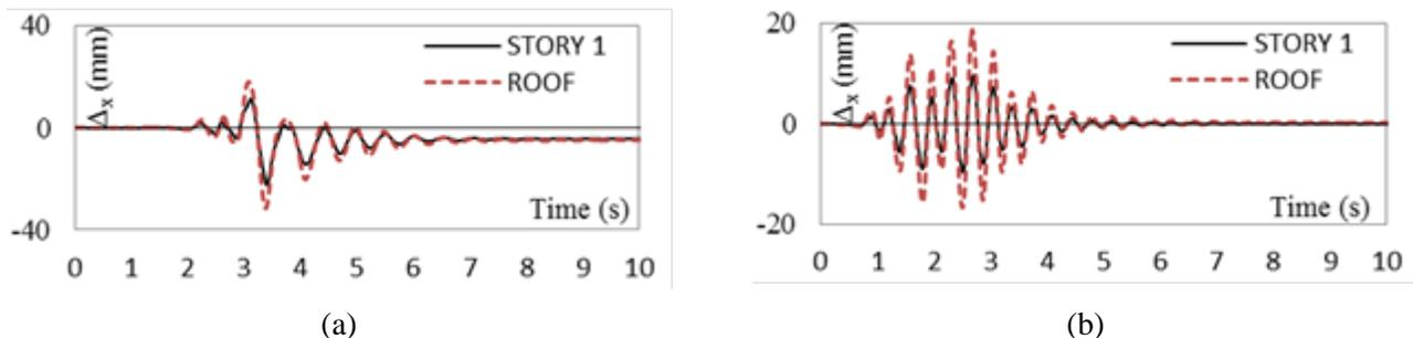
Fig. 5 – Buildings displacement time histories under seismic event 5, (a) displacement in the X direction, (b) displacement in the Y direction
