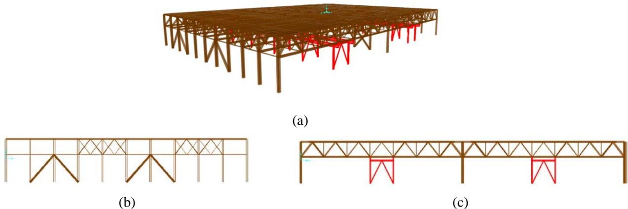
Fig. 1 – Existing Building; (a) 3D illustration from SAP 2000, (b) section along the N-S direction, and (c) section along the E-W direction
