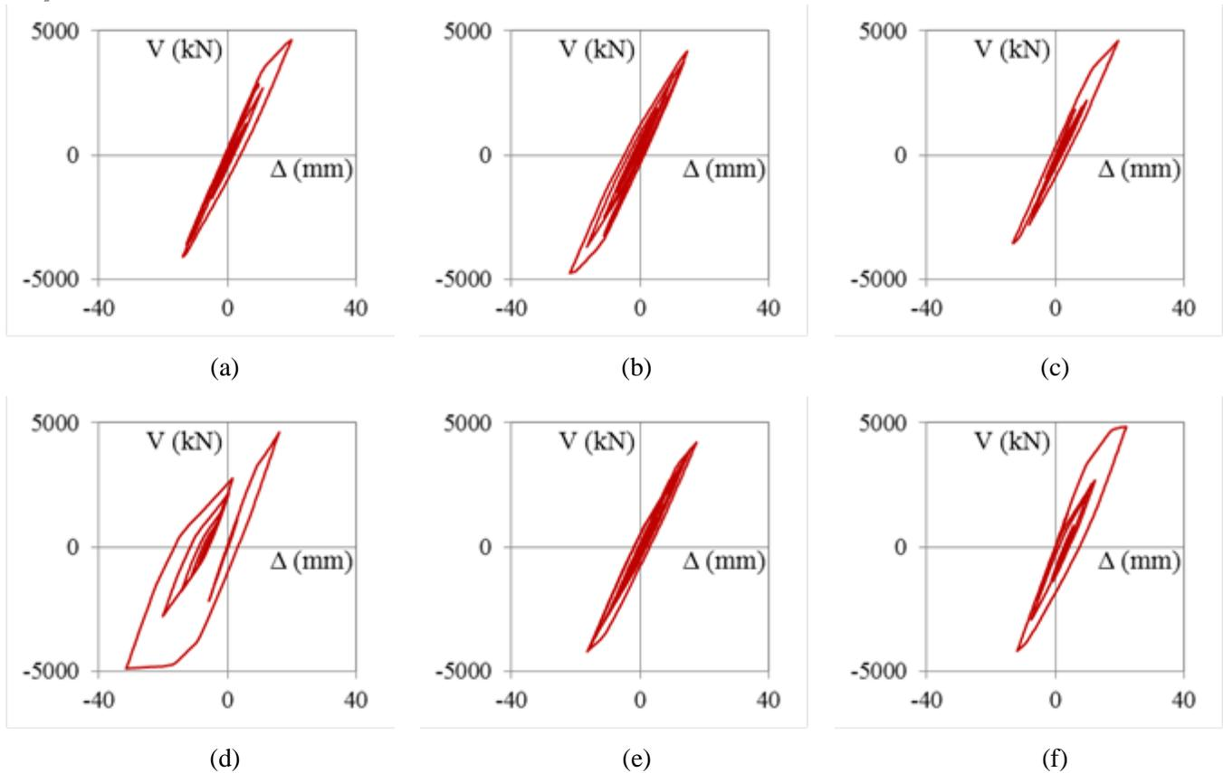
Fig. 6 – Hysteretic response of building II in the X direction subjected to six of the seismic events: (a) event 1, (b) event 2, (c) event 3, (d) event 4, (e) event 5, (f) event 6
