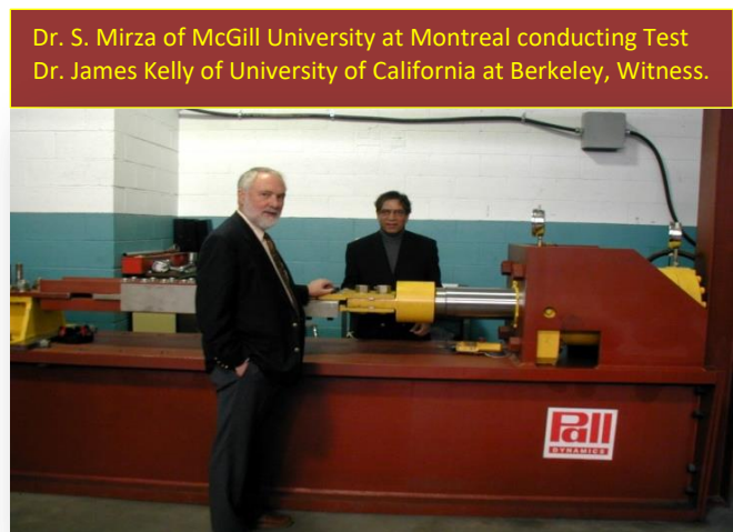
Fig.-14- PDL Test Rig: Capacity 500 Kip / \pm 10'' (Typical) Testing of Pall Friction Dampers
