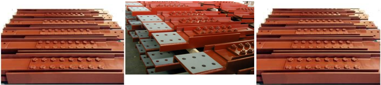
Fig.-16- PFDs laid out after painting for inspection
