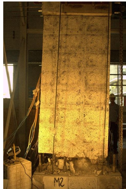
Fig. 6 - Lateral load vs top displacement and fracture Specimen 2
