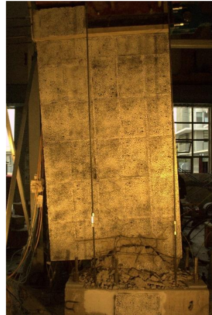
Fig. 7 - Lateral load vs Top displacement and fracture Specimen 3
