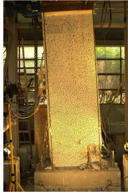
Fig. 5 - Lateral load vs top displacement and fracture Specimen 1
