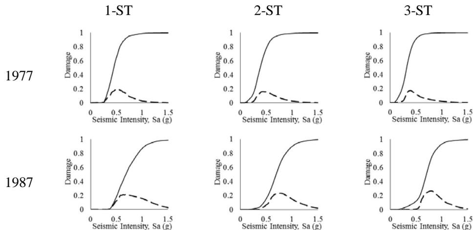
Fig. 7 – Vulnerability curves and its associated standard deviation for the different story structures designed with 1977 and 1987 building codes and retrofitted to accomplish with the 2004 Mexico City building code for one story (1-ST), two stories (2-ST) and three stories (3-ST)
