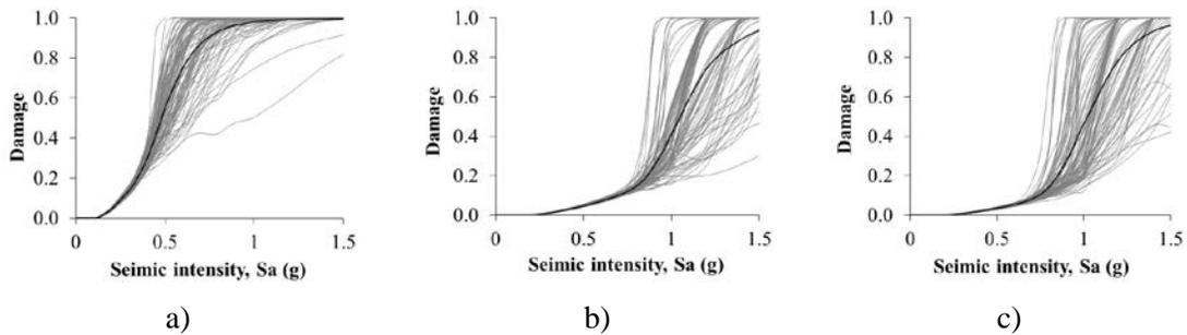
Fig. 4 – Expected damage for three-story structures designed according to: a) 1977, b) 1987 and c) 2004 Mexico City Building Codes
