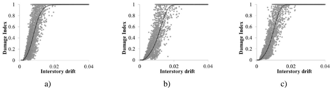
Fig. 3 – Damage Index (Eq. 1) vs. Interstory drifts relationship of a SDOF systems representing three-story buildings according to: a) 1977, b) 1987 and c) 2004 Mexico City Building Codes
