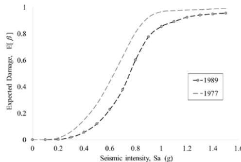
Fig. 5 – Vulnerability curves of retrofitted three-story buildings to accomplish with 2004 building code
