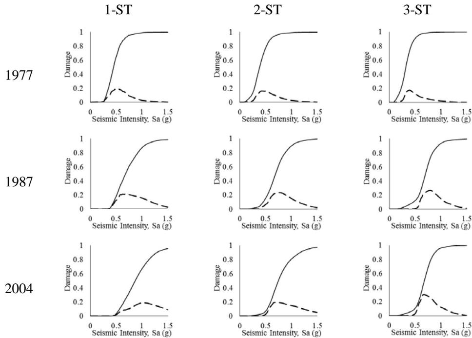
Fig. 6 – Vulnerability curves and its associated standard deviation for the different story structures and different Mexico City building codes for one story (1-ST), two stories (2-ST) and three stories (3-ST)
