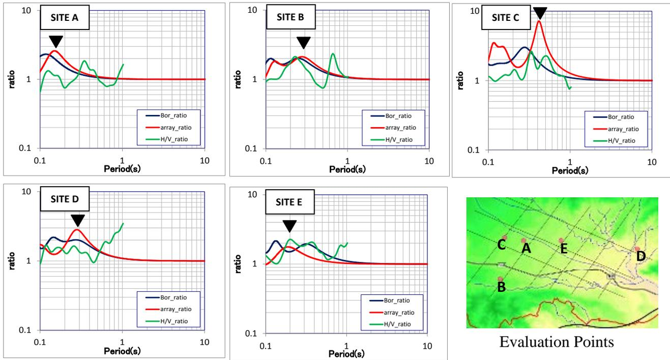
Fig. 6 Transfer functions obtained from boring and miniature arrays (SIM) and H/V spectral ratio
