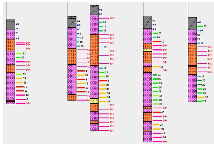
Fig. 3 Example of boring histogram (simple histogram)
