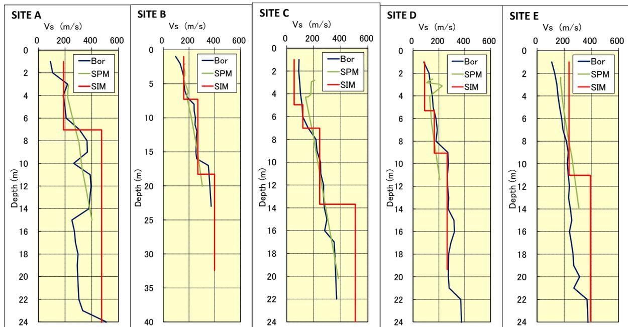
Fig. 5 S-wave velocity structure determined from boring (Bor) and miniature arrays (SPM and SIM)
