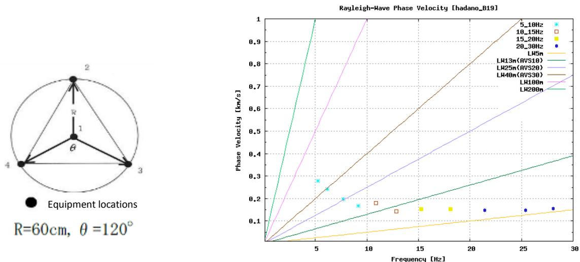
Fig. 4 Positioning of miniature array and an example of phase velocity obtained from results (site B)
