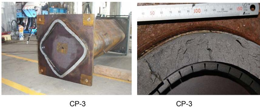
Fig. 7 – Photos of the fractured specimen
