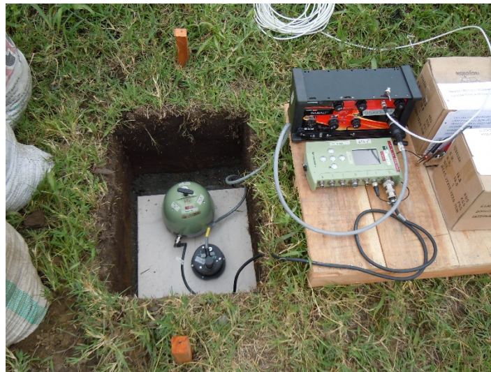
Figure 5. Seismological and accelerographic station installed on the ground to record microtremor.
