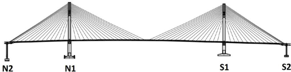
**Fig. 2: Simplified elevation of Port Mann Bridge**
