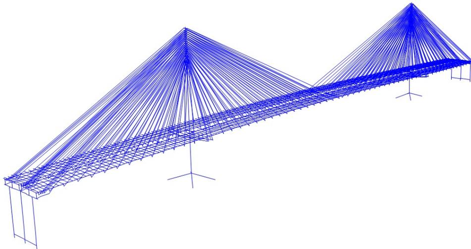
**Fig. 5: Finite element model in SAP2000**
