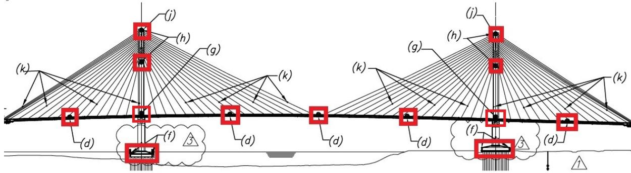
**Fig. 3: Location of sensors used for experimental data**
