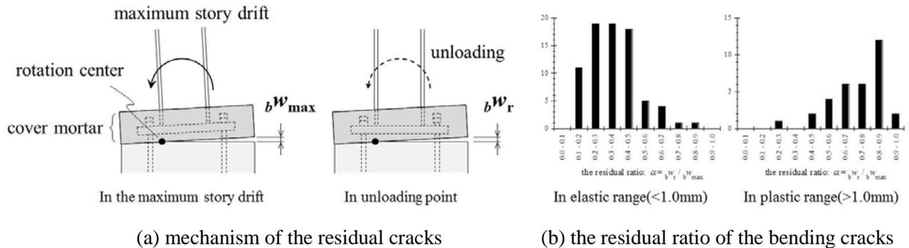
Fig. 8 – Mechanisms of the residual bending cracks and the residual ratio of bending cracks
