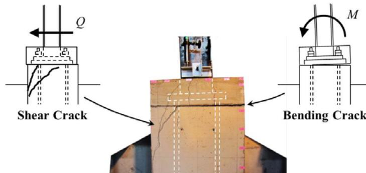
Fig. 7 – The major severe cracks on the concrete foundation around the steel column base
