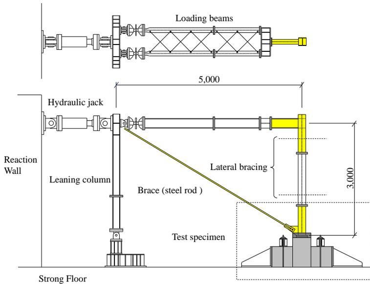
Fig. 2 – Experiment setup (unit :mm)
