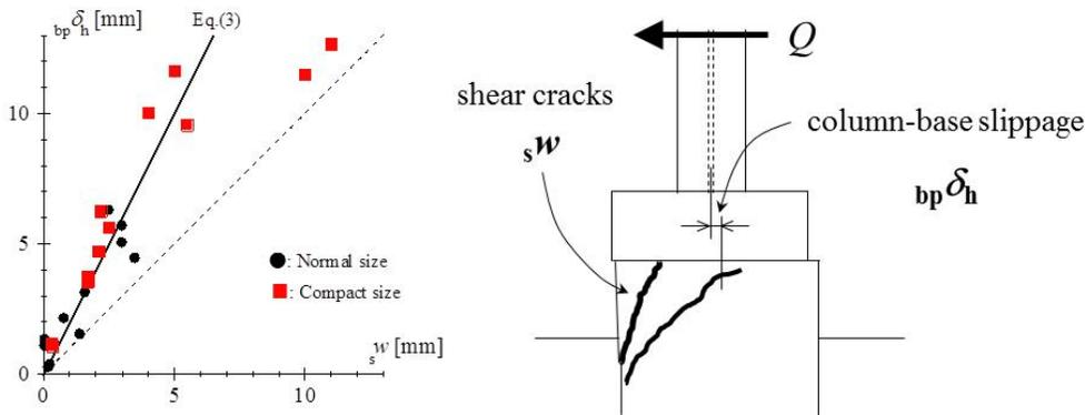
Fig. 10 – Relationships between the maximum width of the shear cracks and column-base slippage
