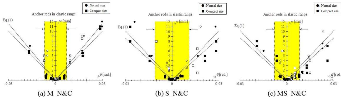
Fig. 9 – Relationships between the maximum and residual width of the bending cracks and column-base rotation
