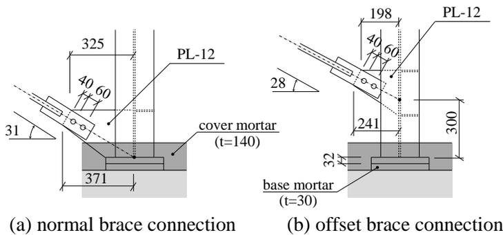
(a) normal brace connection (b) offset brace connection
