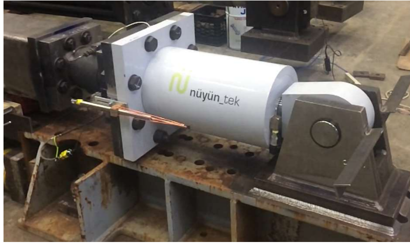
Fig. 5 – Damper connected to the test rig at ATLSS Engineering Research Center at Lehigh University in Bethlehem, USA.
