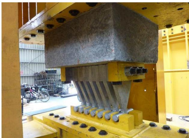
(a) Prototype Building A, Type I connection.
