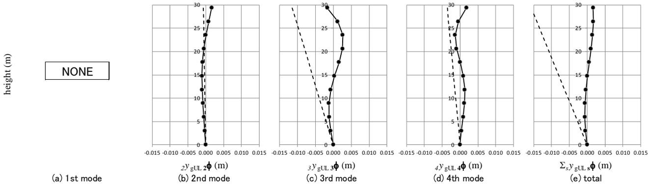
Fig. 9 – Modal displacement vector (at limited equilibrium position)
