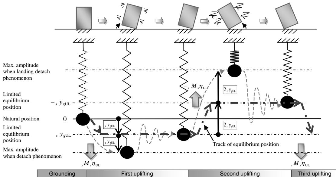
Fig. 4 – Mechanism of generation of higher mode vibration
