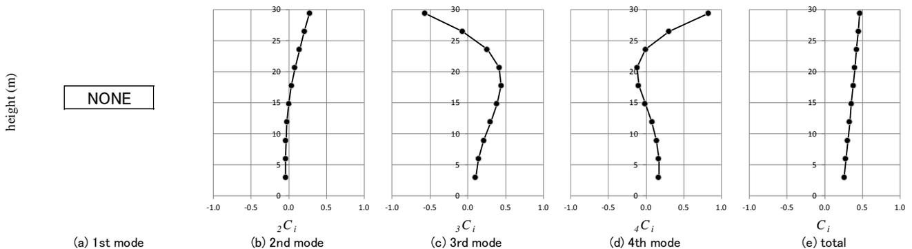
Fig. 10 – Modal shear coefficient (at limited equilibrium position)
