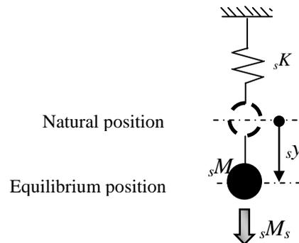
Fig. 3 – Spring pendulum system under pseudo gravity
