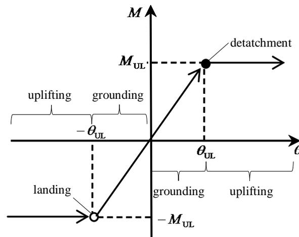
Fig. 12 – The definitions of uplifting, grounding, landing and detachment
