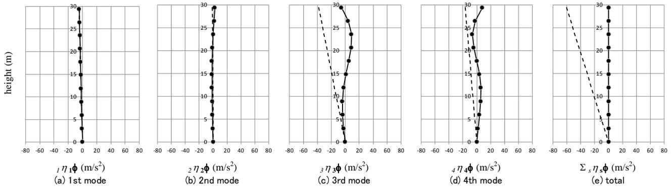
Fig. 8 – Modal gravity acceleration vector
