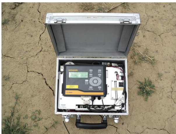
Fig. 4 – (a) Observed microtremor instrument and (b) Shape of the performed array measurement
