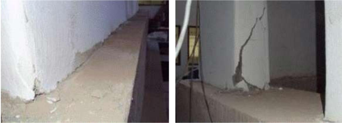
Fig. 12- Damage to the model reinforced after the test.
