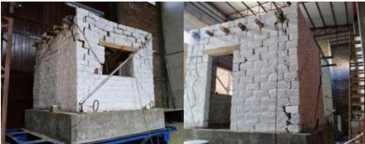
Fig. 11- Model without reinforcement collapsed.
