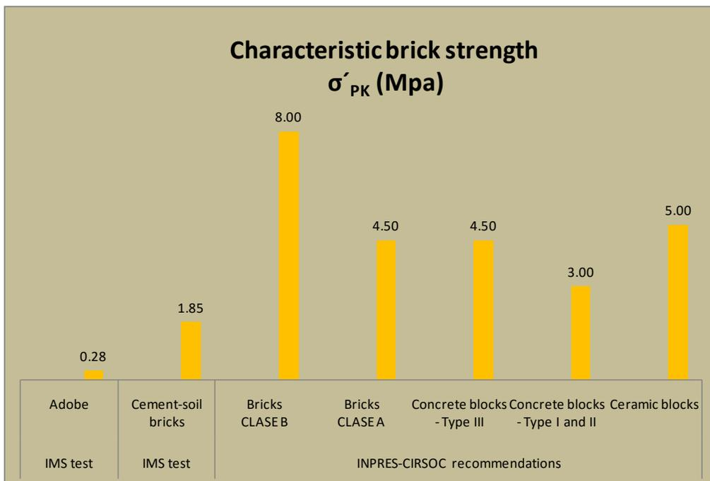
Fig.2-Compressive strength of different bricks<sup>2</sup>
