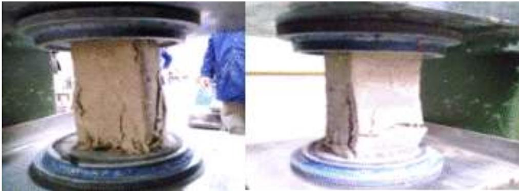
Fig.1- Failure mechanism in compression test.
