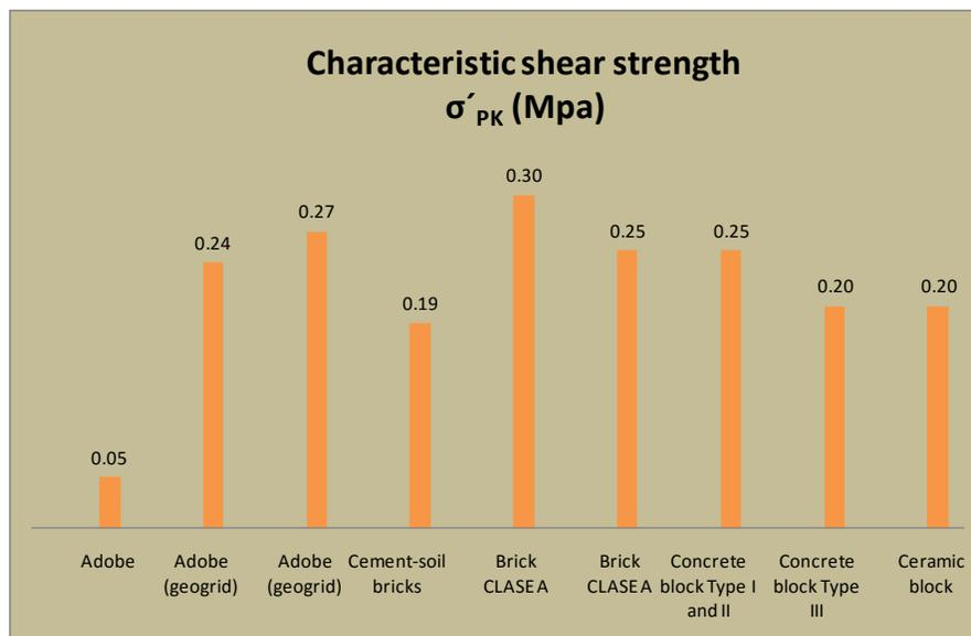
Fig.6-Characteristic shear strength of different types of masonry.
