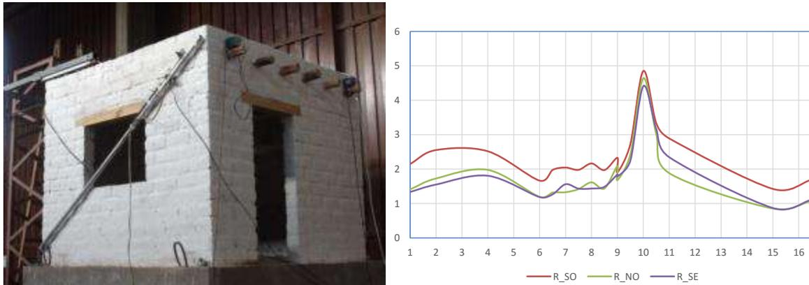
Fig. 10- Model without reinforcement. Resonance curve.
