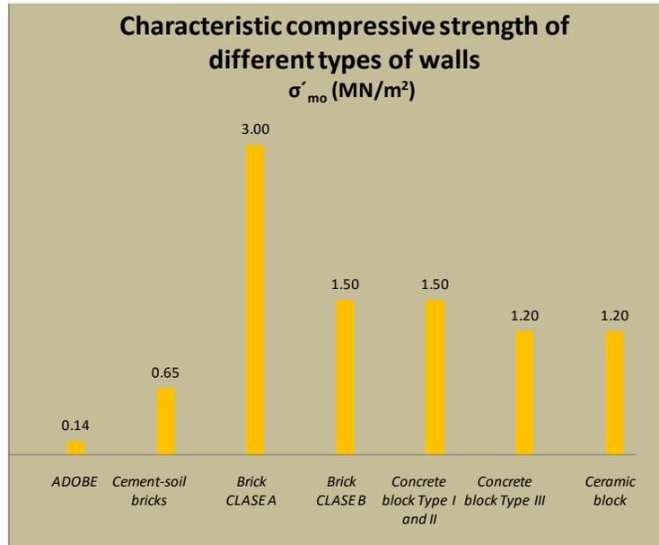
Fig.4- Characteristic compressive strength of different types of masonry<sup>5</sup>
