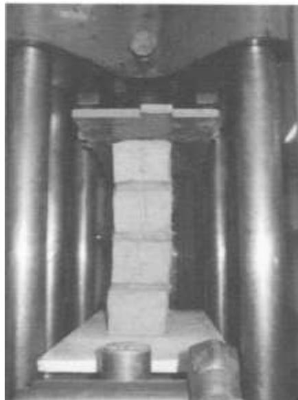
Fig.3- Compressive test on masonry prisms.
