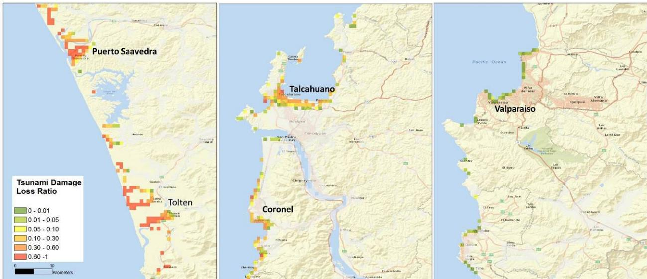
Fig. 6- Loss ratio for tsunami damage at 1km grid cells
