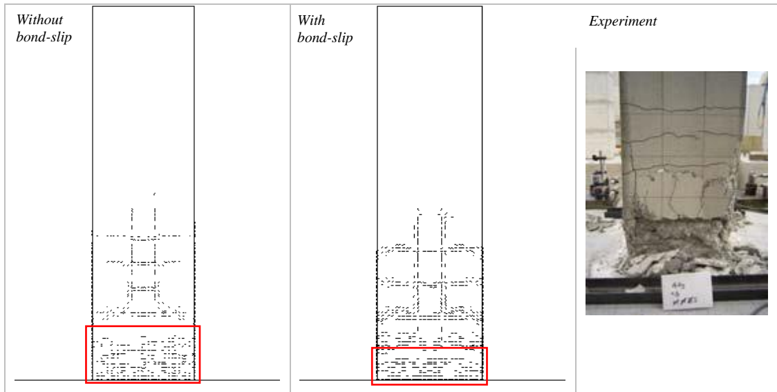
Figure 9 – Comparison of crack patterns of V4
