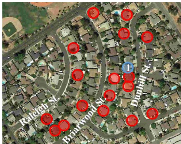
Fig. 5 – Aerial view of Fire Station area depicting homes on three streets having chimneys damaged by the Yountville earthquake (denoted by circles). Investigation shortly after the South Napa earthquake found only one damaged chimney (denoted by “1” in the image).
