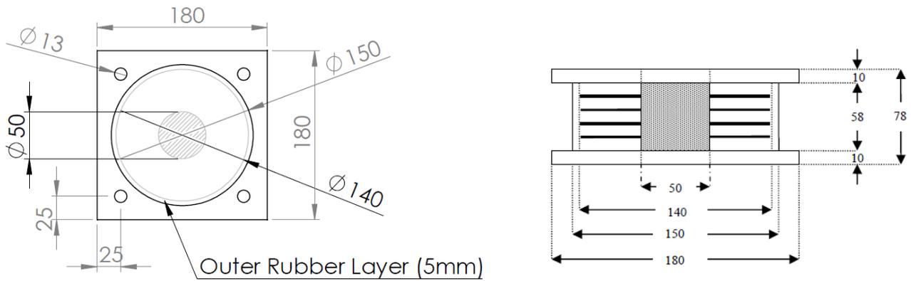
Figure 2. Lead Rubber Bearing Design Details
