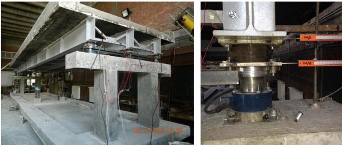
Figure 3. Test Bridge and Bridge Bearings
