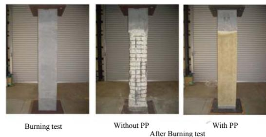
Figure 15. Fire resistance experiment
