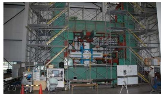
Figure 14. Beam-column joint experiment
