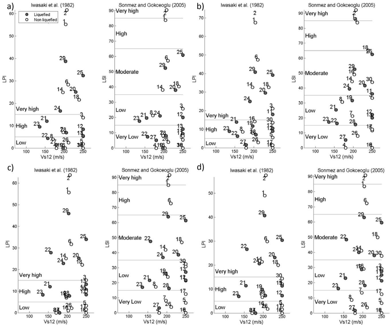
Fig. 3 – Liquefaction potential and severity index: (a) NCEER ws [2]; (b) Cetin et al [3]; (c) Idriss and Boulanger [4]; (d) Boulanger and Idriss [5].
