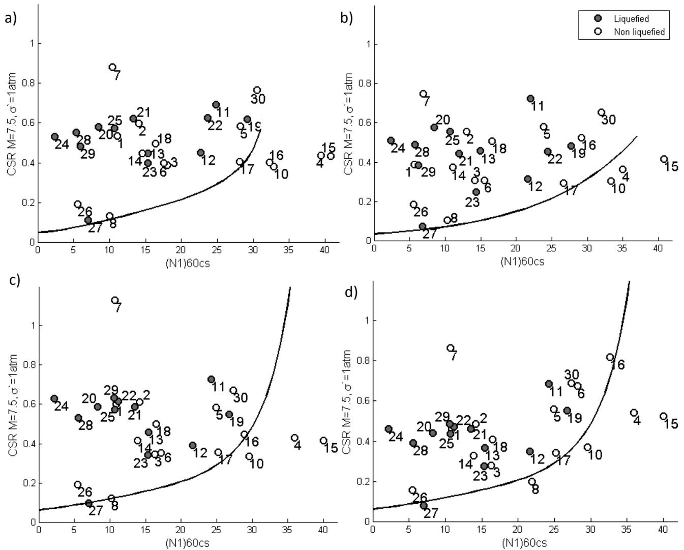
Fig. 2 – Liquefaction triggering analysis using PGA as demand proxy. (a) NCEER ws [2]; (b) Cetin et al [3]; (c) Idriss and Boulanger [4]; (d) Boulanger and Idriss [5].
