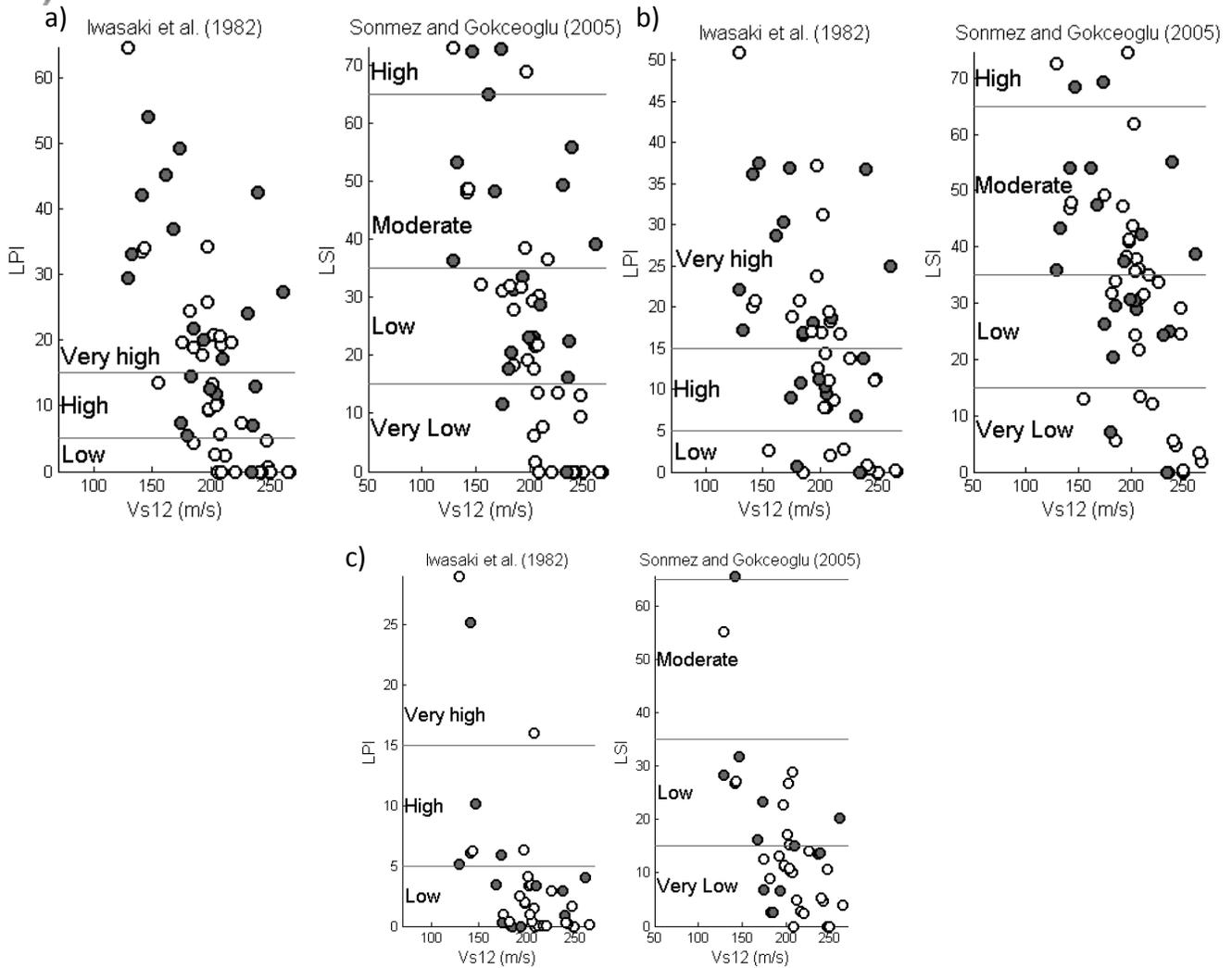
Fig. 5 – Liquefaction potential and severity index: (a) Andrus et al. [6]; (b) Kayen et al. [7]; (c) Dobry and Abdoun, [8].
