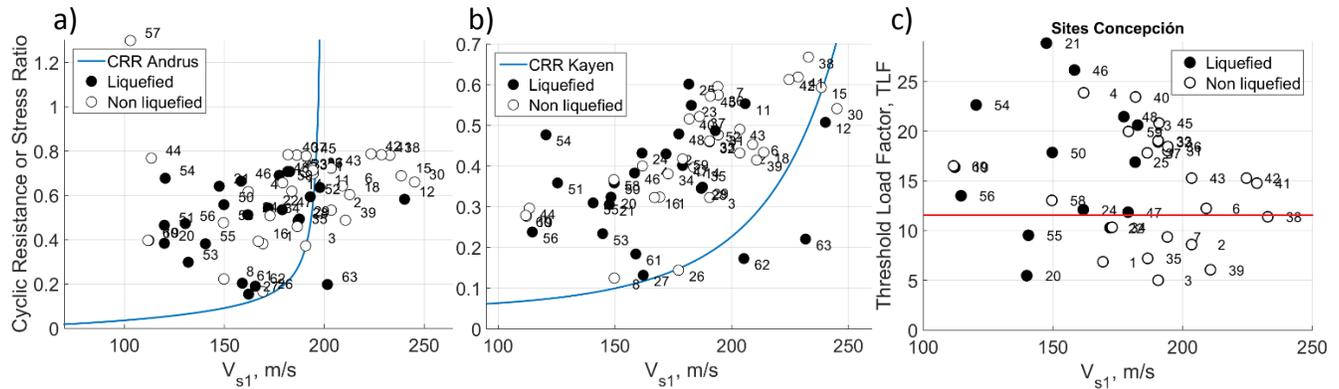
Fig. 4 – Liquefaction triggering analysis using PGA as demand proxy: (a) Andrus et al. [6]; (b) Kayen et al. [7]; (c) Dobry and Abdoun, [8]. Blue lines are the deterministic boundary proposed by each methodology, and the red line for [8] is a preliminary estimation of the division of classes made by the authors.
