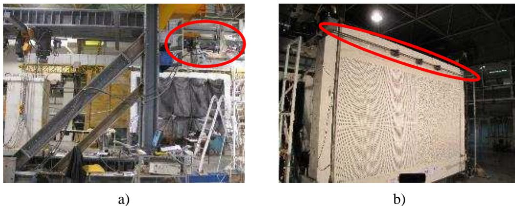
Fig. 12 – Detail of: a) Servo-controlled hydraulic actuator ( $\pm 500\text{kN}$  capacity with  $\pm 150\text{mm}$  stroke) attached to a reaction steel frame; and b) horizontal high-strength rods ( $\phi 30\text{mm}$ ) that are connected to the left and right steel profile placed at mid-height of the top beam.
