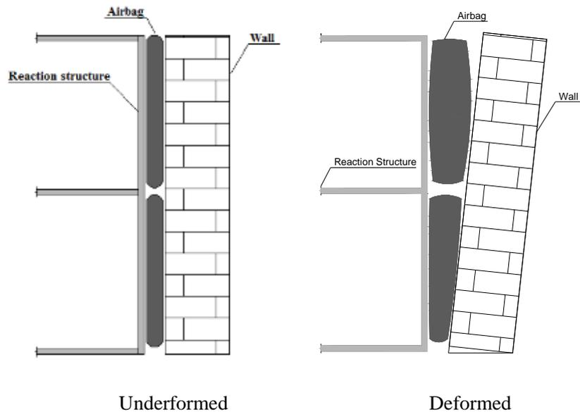
Fig. 5 - Variation of the contact area for extreme displacement situations
