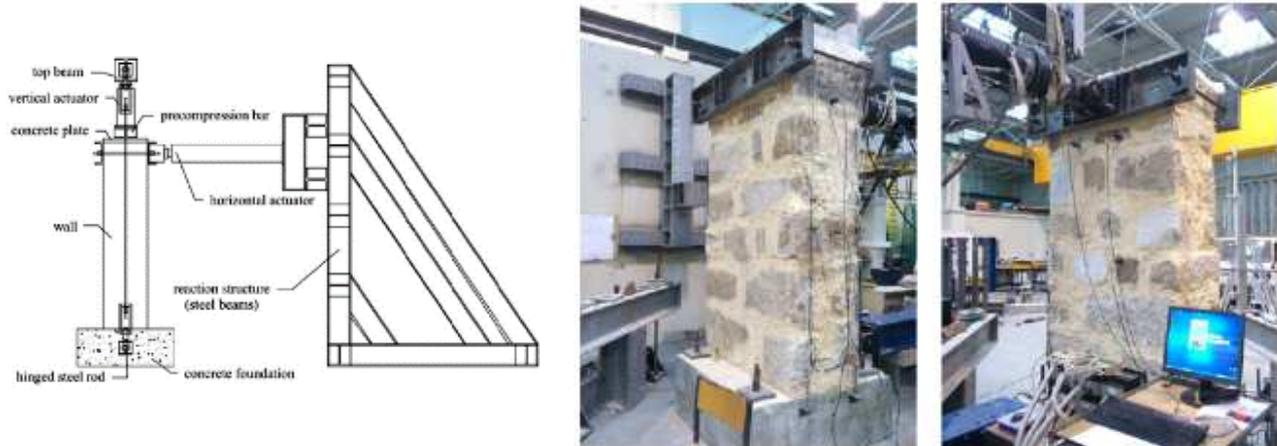
Fig. 8: Out-of-plane point load test setup implemented in the Laboratory of Earthquake and Structural Engineering.
