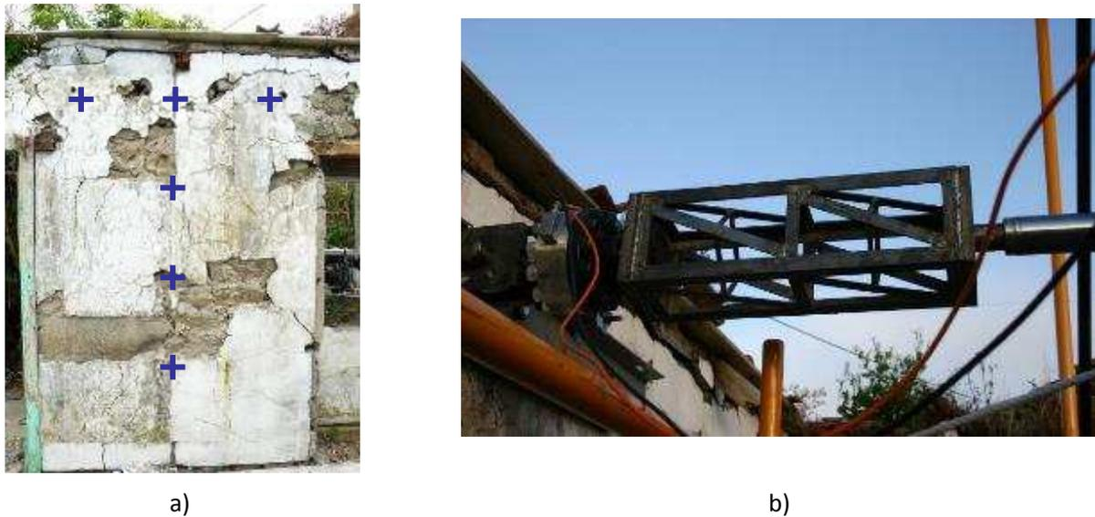
Fig. 3 - Measurement details: a) layout of displacement measurement; b) load cell.
