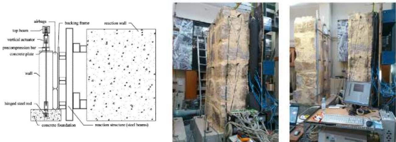
Fig. 7: Out-of-plane distributed loads using airbags test setup implemented in the Laboratory of Earthquake and Structural Engineering.
