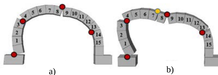
Fig. 12 – Collapse mechanism during quasi-static analysis (structure tilted from the left side) as the collapse a) was initiated and b) as it progressed
