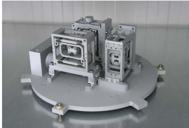
Fig. 5 – Triaxial Folded Pendulum Seismometer/Accelerometer - xyz configuration.
