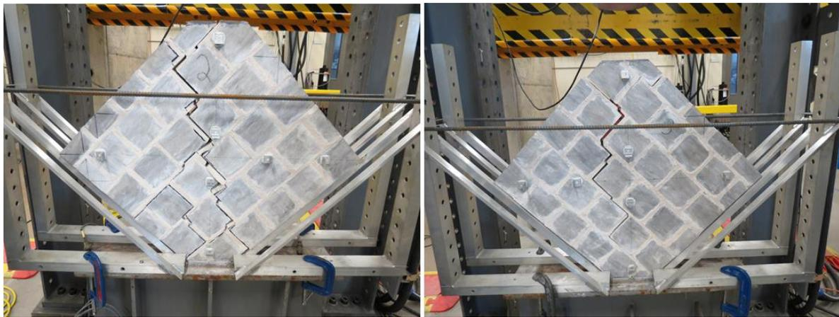
Fig. 7 – Failure pattern at the end of the diagonal shear tests on stone masonry panels.
