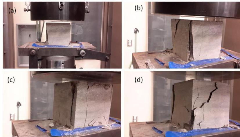
Fig. 2 – Compression tests on limestone: (a) Test setup; (b), (c) and (d) Failure mechanism for the three tested stone cubes.
