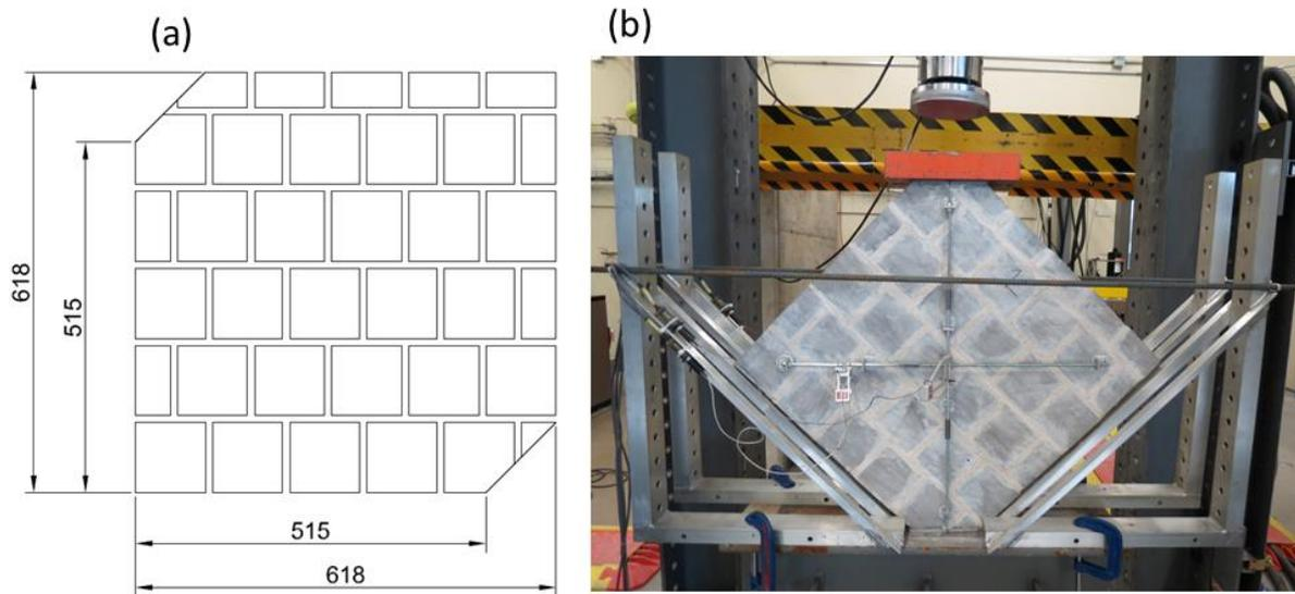
Fig. 6 – Diagonal shear tests on stone masonry panels: (a) panel dimensions (mm) and (b) test setup.
