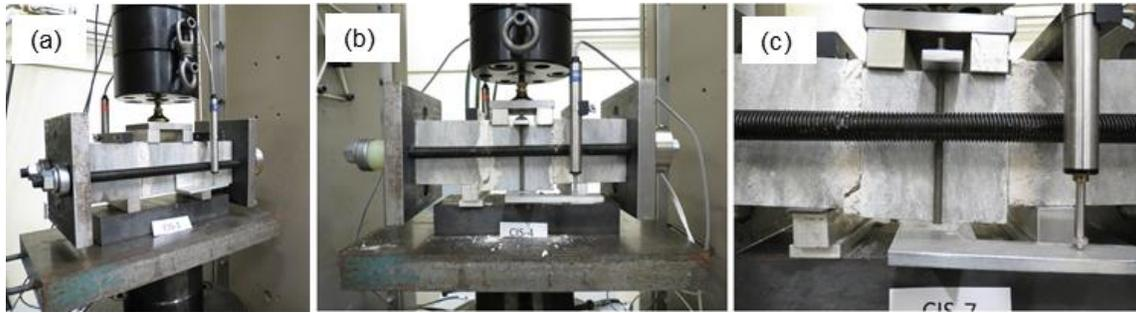
Fig. 4 – Masonry joint shear bond tests: (a) Test setup; (b) and (c) crack pattern at the end of the tests.
