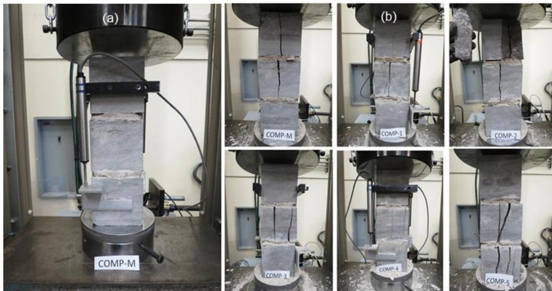
Fig. 3 – Masonry compression tests: (a) Test setup; and (b) crack pattern at the end of the tests.
