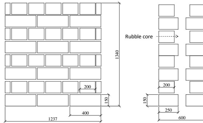
Fig. 1 – Elevation (left) and cross-section (right) of a representative three-leaves stone masonry wall.
