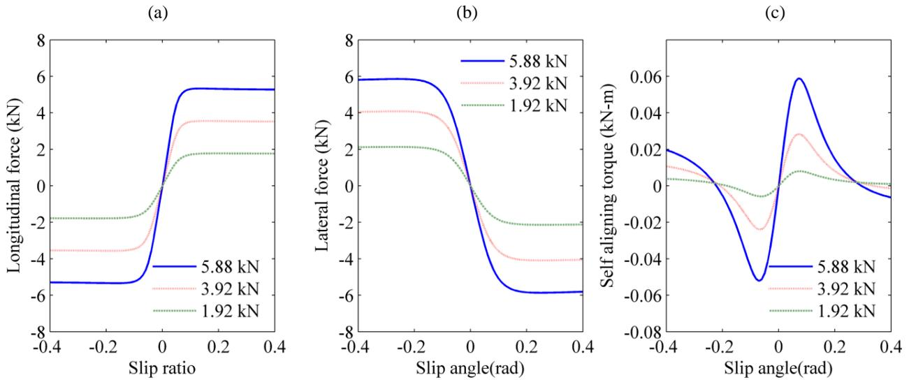
Fig. 5 – Relationship of longitudinal and lateral forces and self-aligning torque with slip ratio and slip angles using Magic Formula Model
