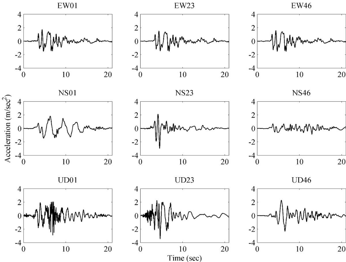
Fig. 3 – Interpolation of earthquake motion for a vehicle with speed 20 m/sec depends on location
