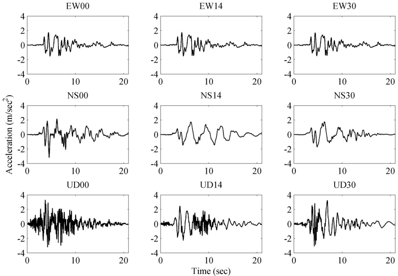
Fig. 4 – Interpolation of earthquake motion for different speed of vehicle
