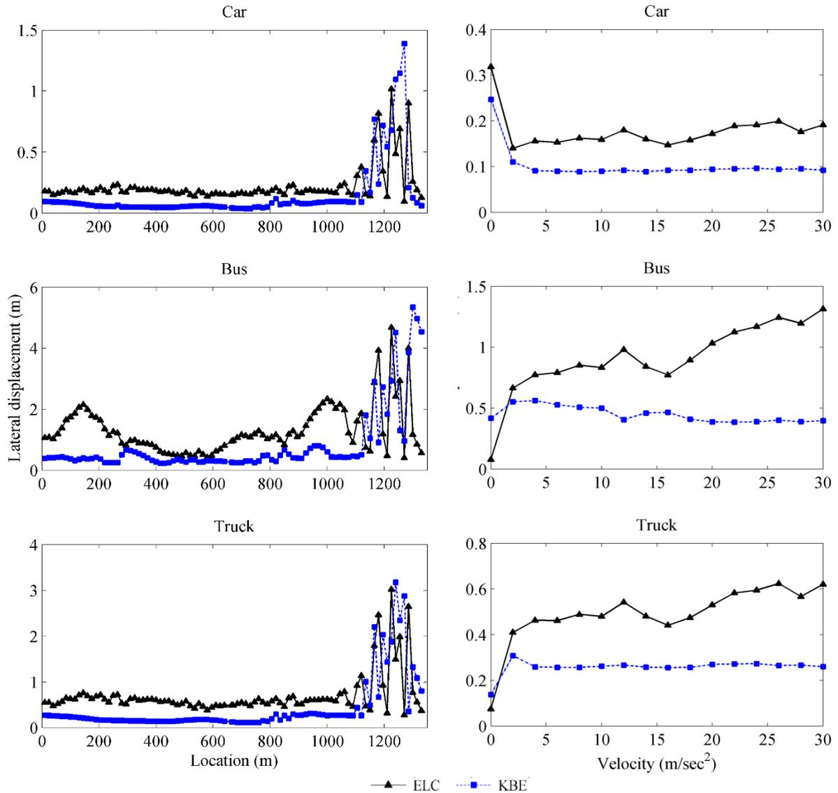
Fig. 6 – Lateral displacement of vehicles for different locations of origin and different speed
