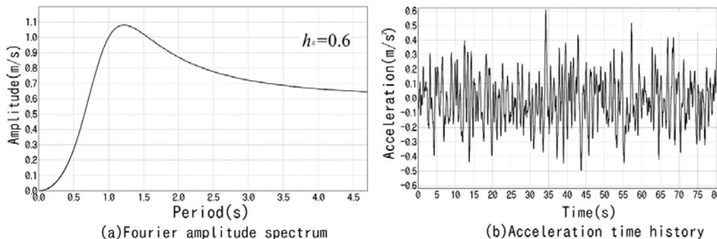
Fig. 4 – Artificial ground motion
