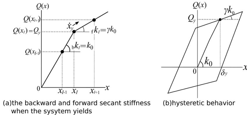
Fig. 2 – Bi-linear restoring force characteristic
