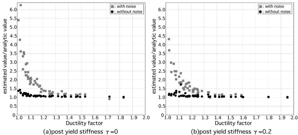
Fig. 7 – Relationship between ductility factor and estimation accuracy
