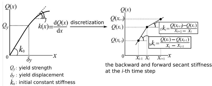
Fig. 1 – The stiffness of discrete data
