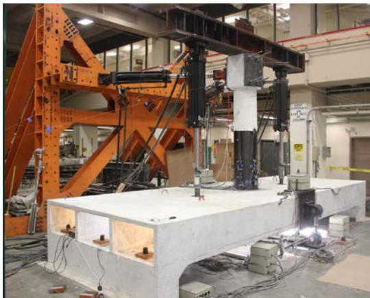
Fig. 10 – MDOF HS test setup using the repaired SP1 bridge subassemblage
