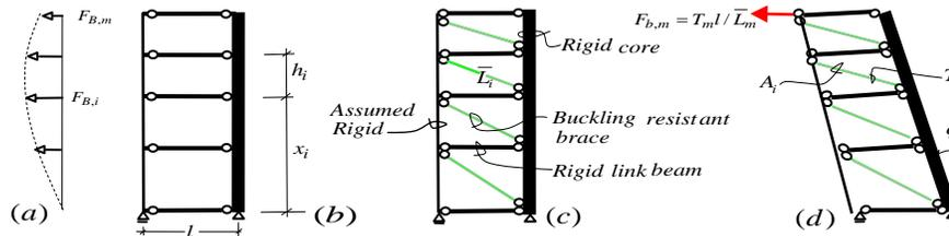
Fig. 3 (a) Notional load, (b) Imaginary mechanism, (c) Braced frame, (d) Rigid body displacement
