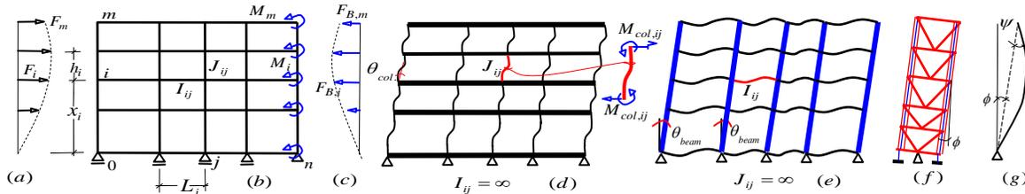
Fig. 2 (a) Loading, (b) GBSMF with gap opening moments, (c), Reactions due to BRBs, (d) GBSMF with rigid beams,(e) GBSMF with rigid columns, (f) Tilted RRC, (g) Deformation of the combined structure.
