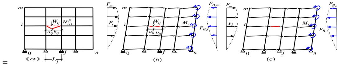
Fig. 4 (a) Beam mechanisms, (b) Mixed (combined, beam +sway) mechanisms, (c) Purely sway mechanism
