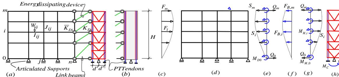
Fig.1 (a) GBSMF with braced RRC and supplementary devices, (b) Concrete RRC, (c) Lateral loading, (d) GBSMF, (e) Interactive forces and gap opening moments acting on the frame, (f) Assumed BRB reactions, (g) Interactive forces and gap opening moments acting on the RRC, (h) RRC base restoring moment.
