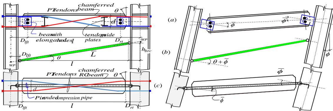
Fig.6 (a) Chamfered steel LB, (b) BRB (c) Chamfered reinforced concrete LB before and after rotation
