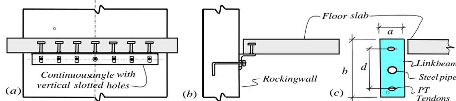
Figure 7(a) Symbolic wall-slab shear connection, (b) Section showing same, (c) Link beam section
