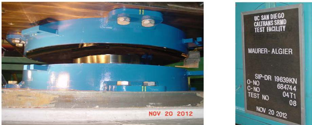
Fig. 10 - Prototype isolators installed into CALTRANS test rig in San Diego
