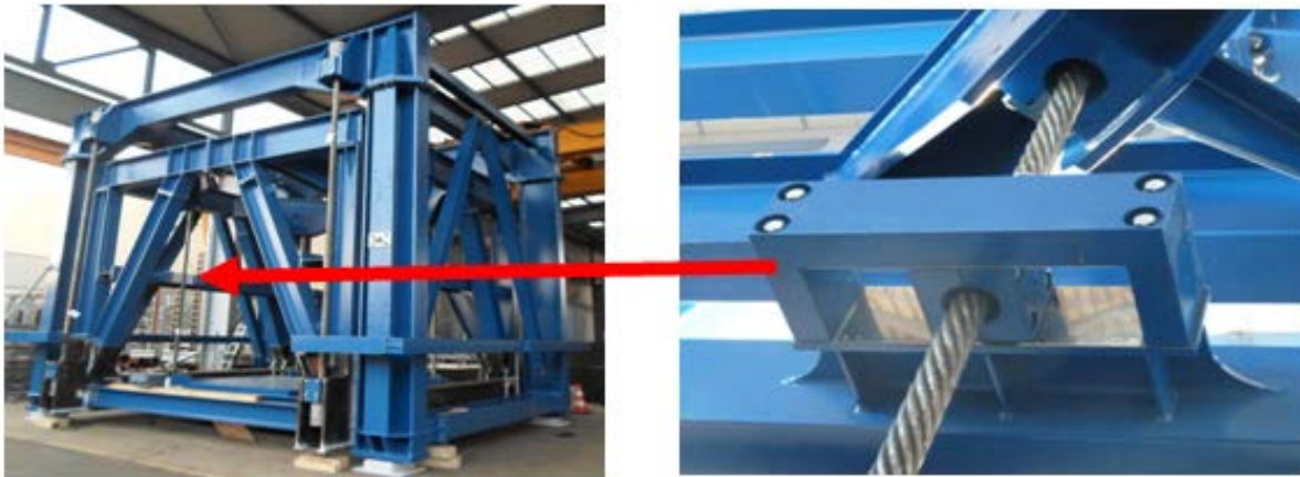
Fig. 5 - Double pendulum steel frames with sliding fixation shoe for various pendulum frequency adjustments in X- and Y-direction.
