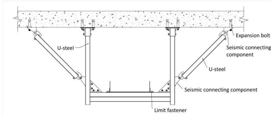
Fig. 2 –Construction of seismic bracing
