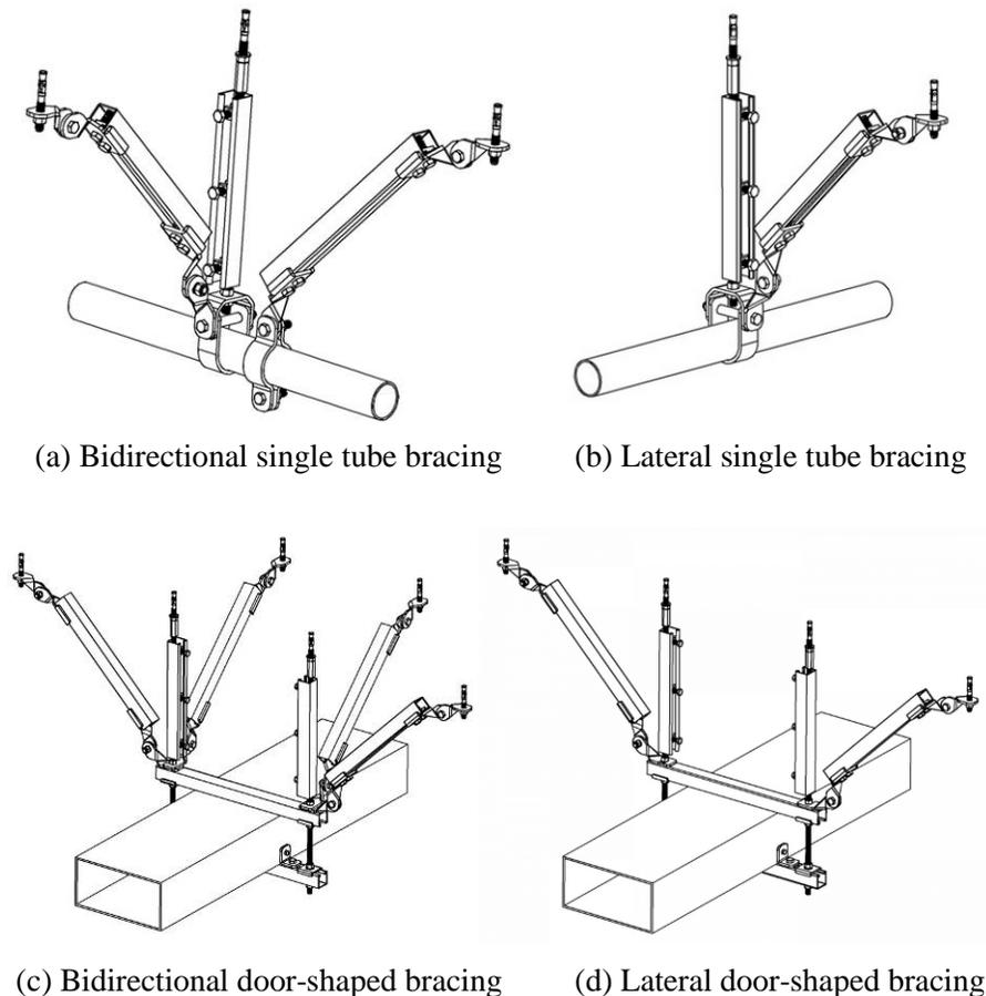
Fig. 1 –Types of seismic bracing
