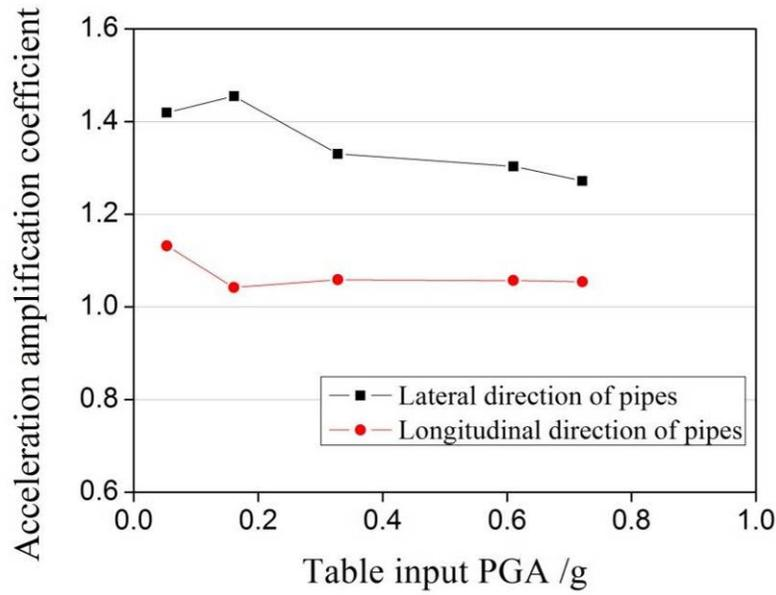
Fig. 6 –Acceleration amplification coefficient of pipes
