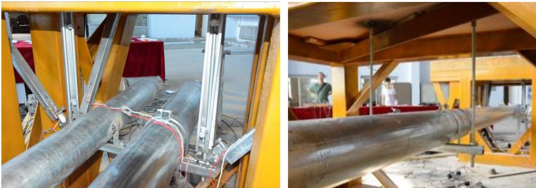
(a) Seismic bracing
