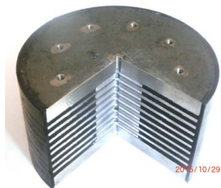
Fig. – 9 Internal view of a tested ARB specimen after more than 200 cycles of loadings
