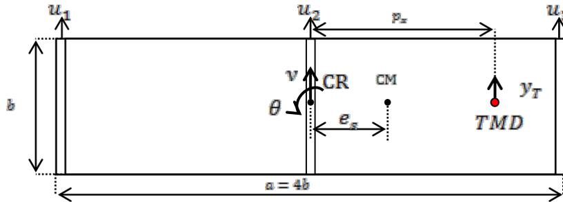
Fig. 1. Mono-symmetric structural model used in the study.
