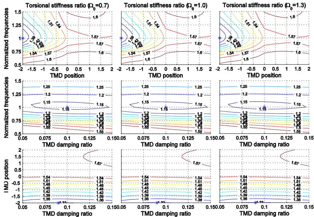
**Fig. 3.** Contour lines of the functional  $J$  for the structure subjected to a BBP ( $T_s = 2.5 \text{ s}$ ,  $e_s/r_s = 0.3$ ,  $\xi_s = 0.05$ ,  $\Omega_s = [0.7, 1.0, 1.3]$ ,  $\mu = 0.02$ ,  $R = 5$ ,  $n = 1$  and  $\alpha_1 = \alpha_2 = \alpha_3 = 0.5$ )
