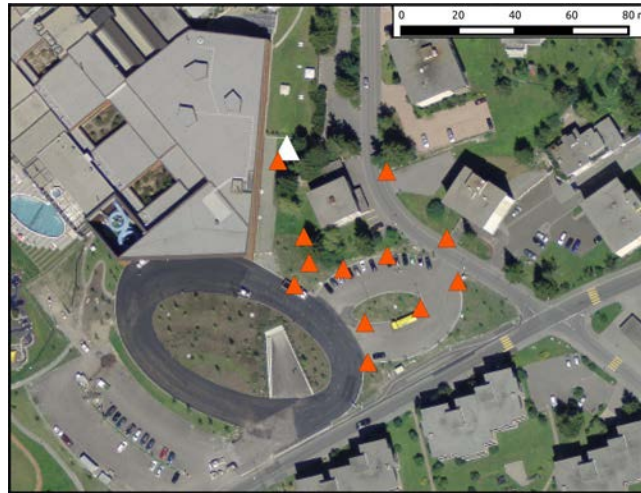
Fig. 5 – Array layout for the passive seismic measurements at station SDAK in Davos. The orange triangles indicate the locations of the seismic sensors in the passive array. The location of site SDAK is indicated by the white triangle. © 2016 swisstopo (JD100042)
