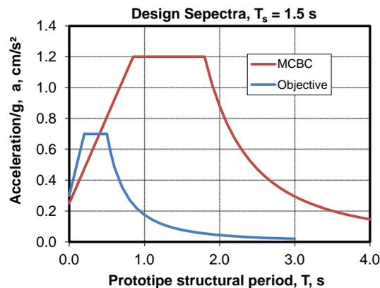
Fig. 5 – Target response spectrum and design spectrum for Mexico City Building Code
