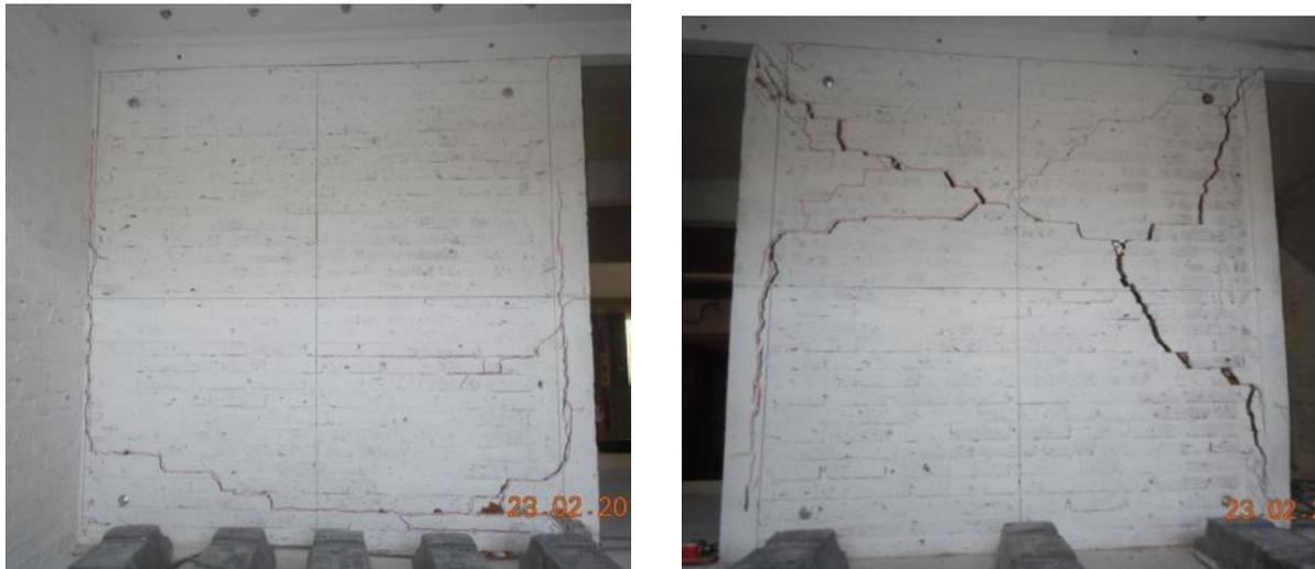
Fig. 8 – Final crack pattern in the Story 2 of specimen M3ND-0, test stage 200%
