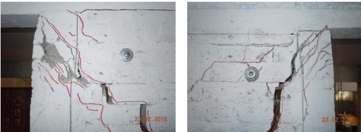
Fig. 9 – Final cracking detail and damage of tie-column at Story 2, specimen M3ND-0
