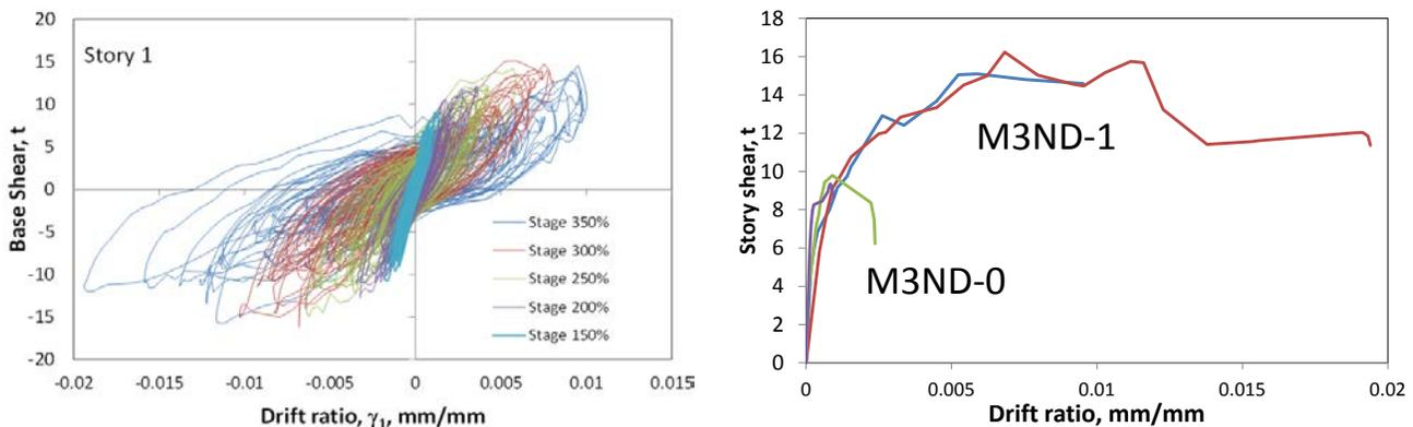
Fig. 12 – Hysteresis curves of M3ND-1, all test stages; and response envelopes of two specimens
