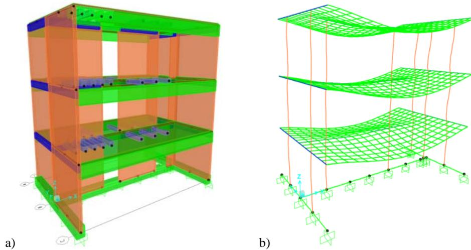
Fig. 4 – Numerical model using wide column method: a) Geometry, b) Deformed shape for gravity load case
