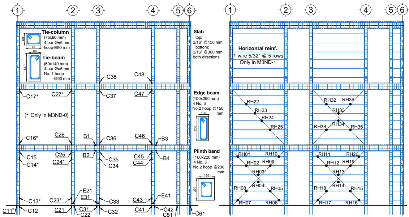
Fig. 2 – Steel reinforcement and strain gauge location; (horizontal reinforcement only in specimen M3ND-1)
