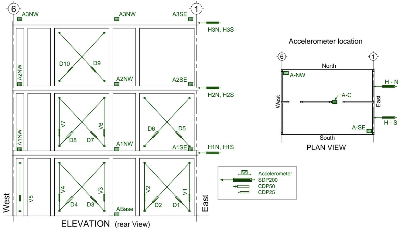
Fig. 3 – External instrumentation and accelerometers
