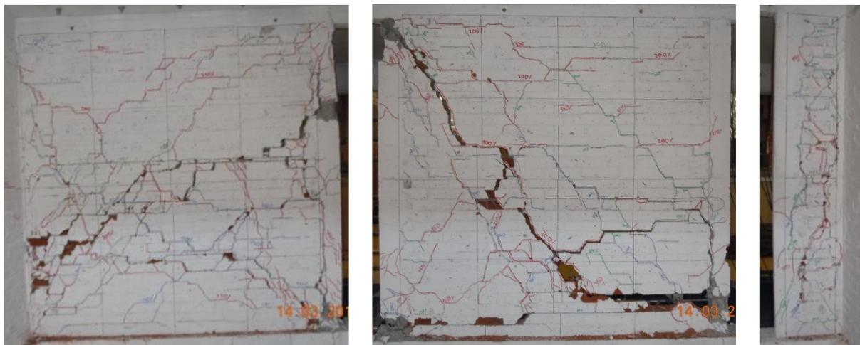
Fig. 10 – Final cracking pattern of Story 1, specimen M3ND-1, test stage 350%
