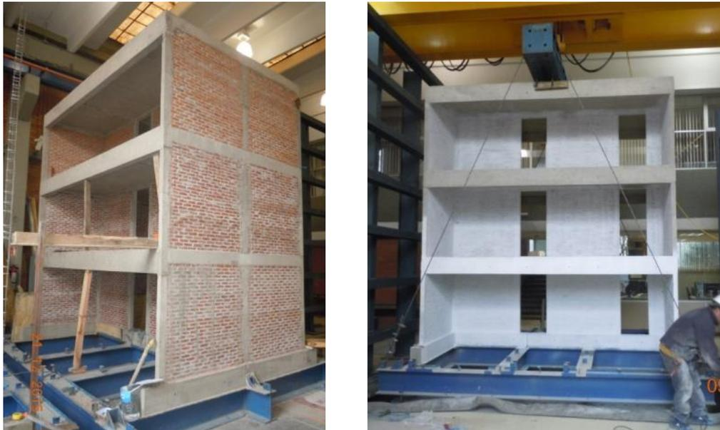
Fig. 7 – Final view of specimen and its movement to the shaking table platform
