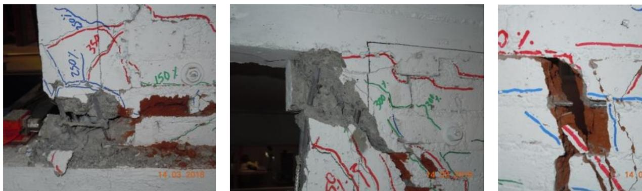
Fig. 11 – Final cracking pattern, detail of tie-column ends and the fracture of horizontal wire
