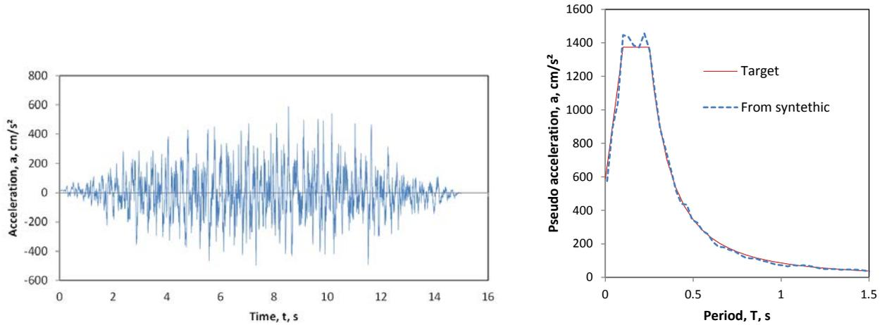
Fig. 6 – Synthetic accelerogram and response spectrum for 5% damping ratio
