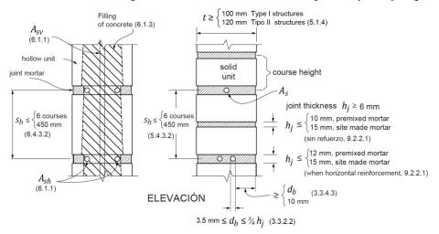
Fig. 2 Position of horizontal reinforcement in masonry walls
