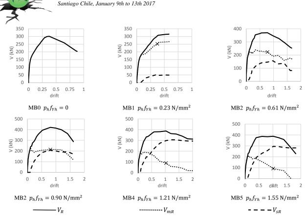
Fig. 3 Contribution of masonry and reinforcement to the wall shear strength [18]
