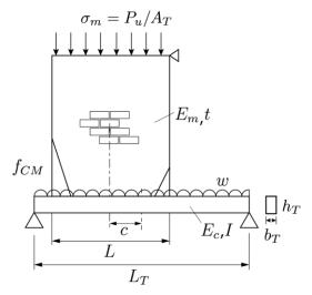
Fig. 1 - Structural wall supported on a beam
