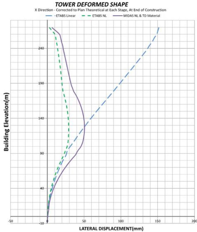
Figure 8 – Lateral Deformation Due to Each Analysis Type
