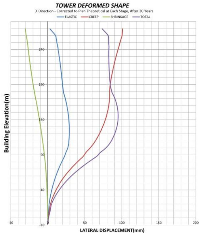
Figure 9 – Lateral Deformation at 30 Years
