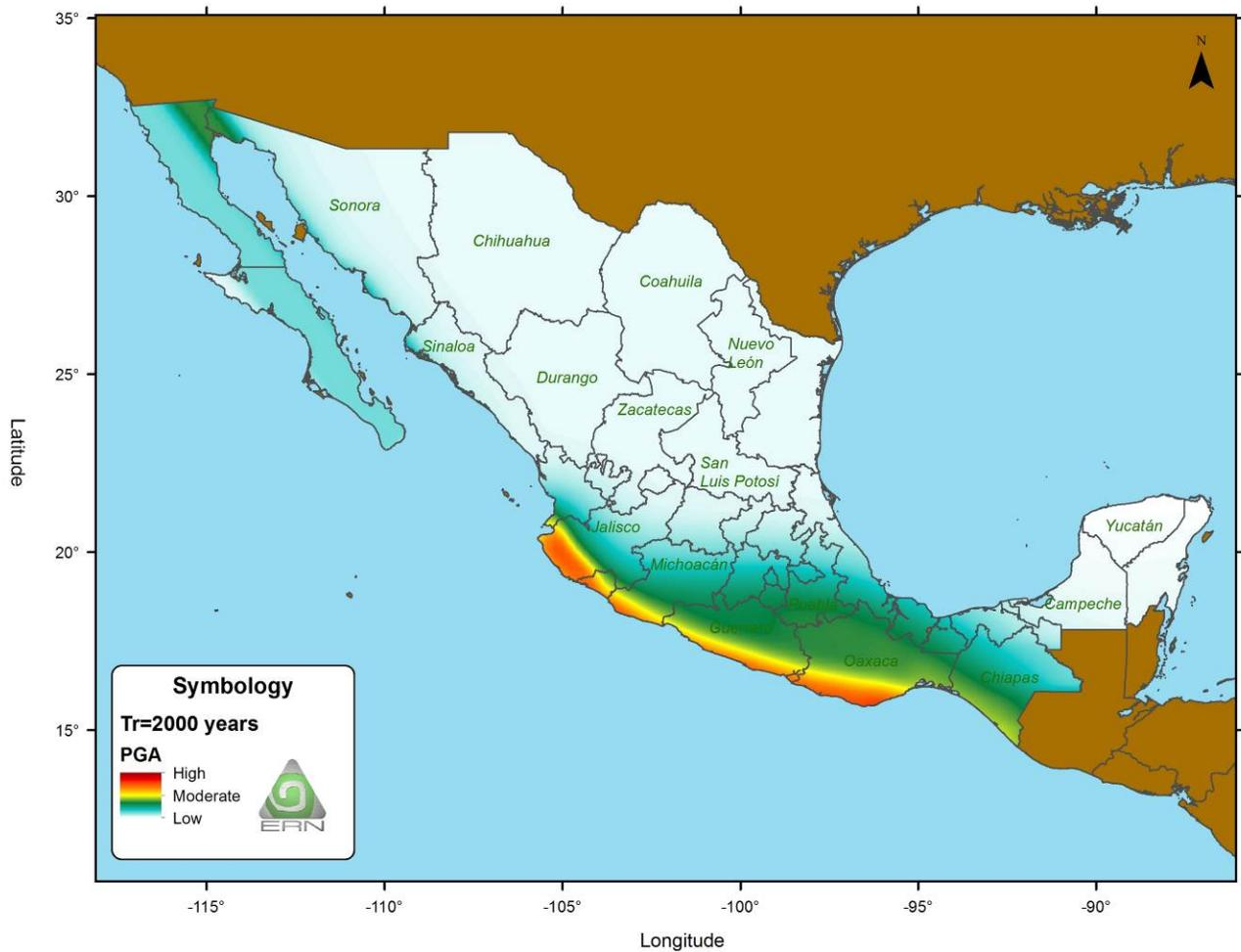
Figure 4 – Seismic Hazard Map of Mexico
