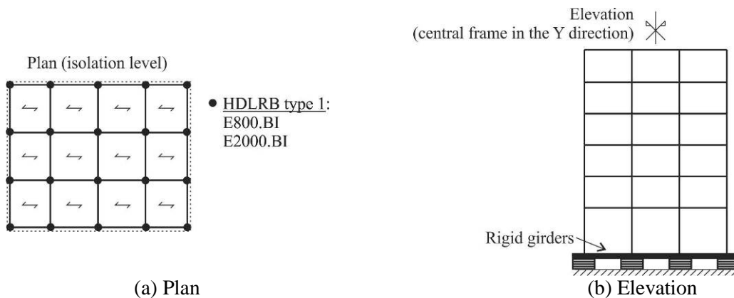
Fig. 3 – EBI structures: HDLRBs type 1 acting alone
