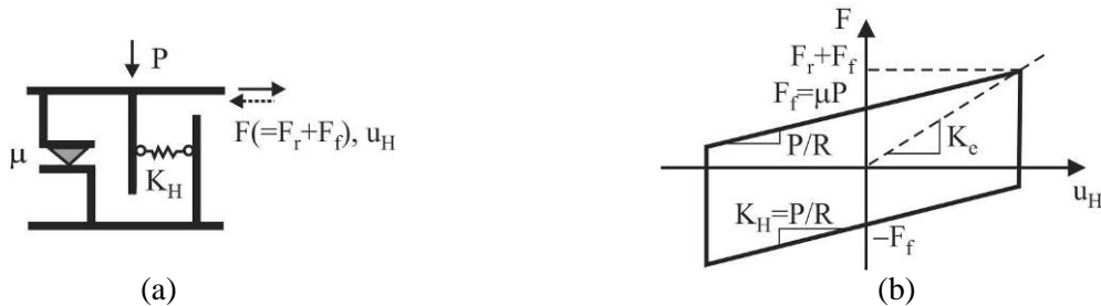
Fig. 8 – Modelling of the base-isolation system for the FPBI structure: FPBs acting alone
