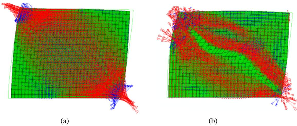
Fig. 4 – Principal stresses at (a) maximum shear and (b) post maximum point. [8]
