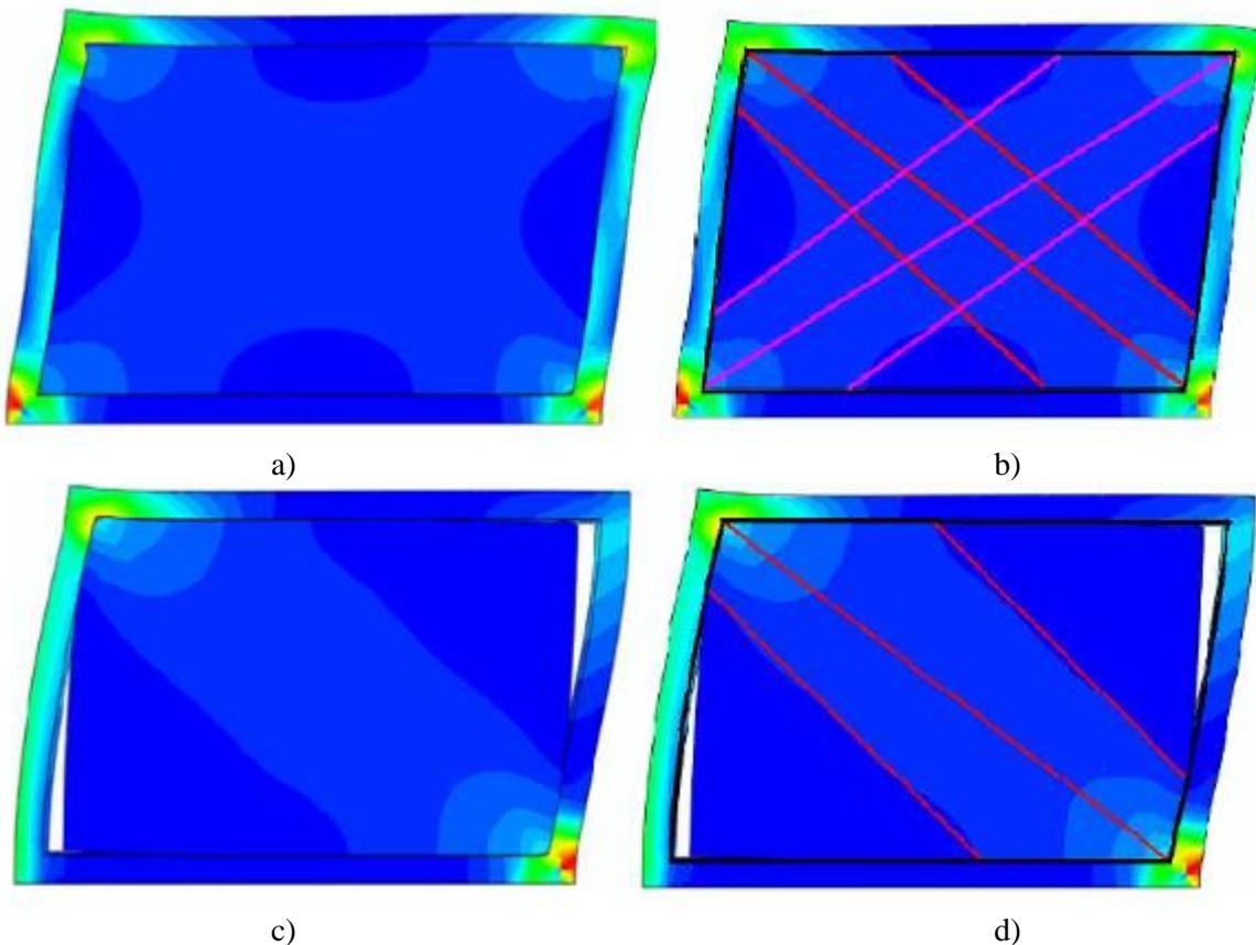
Fig. 3 – Deformed shape and Von Misses stresses in a finite element model of a confined masonry wall (a) at the initial stage, and (b) Initial stage with justification for three struts, c) after separation, d) after separation with struts [8]
