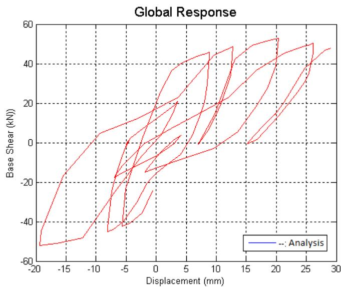
Fig. 14 – Dynamic response of 3D model.
