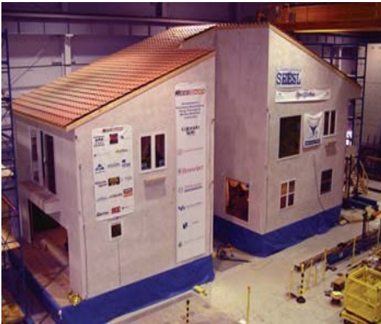
Fig. 2 - Testing of a two-story townhouse at the NEES at Buffalo
