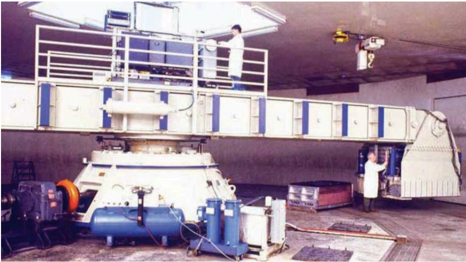
Fig. 6 - The UC Davis centrifuge with the largest radius and platform area in the United States
