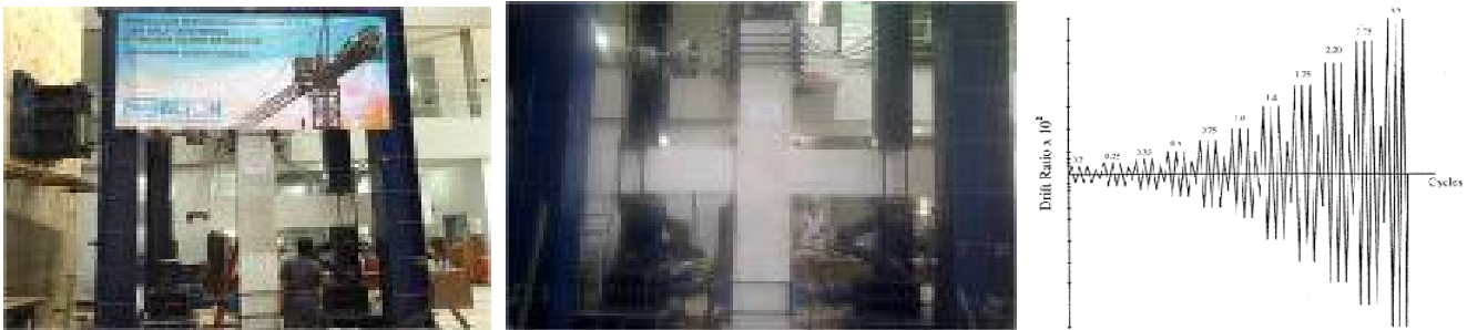
Fig. 16– Beam column joint test
