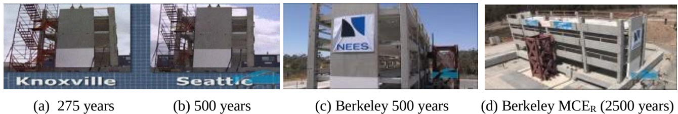
Fig.3 – Testing of high performance earthquake resistant structure with shaking table equipment [17]
