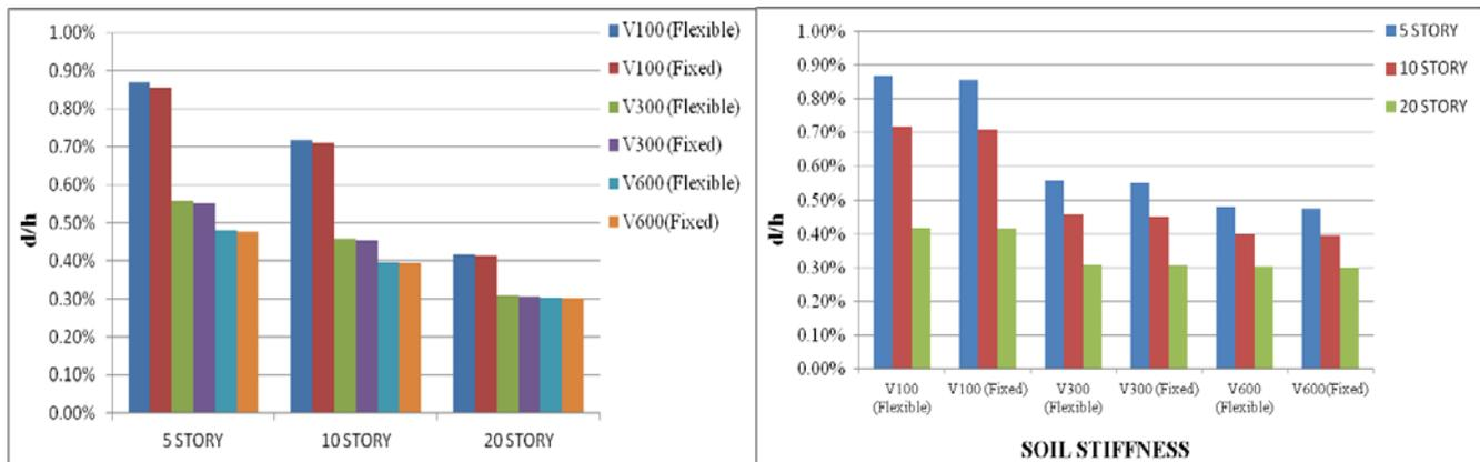
Fig. 8 – Drift ratio (Y direction) of different structures on different support conditions
