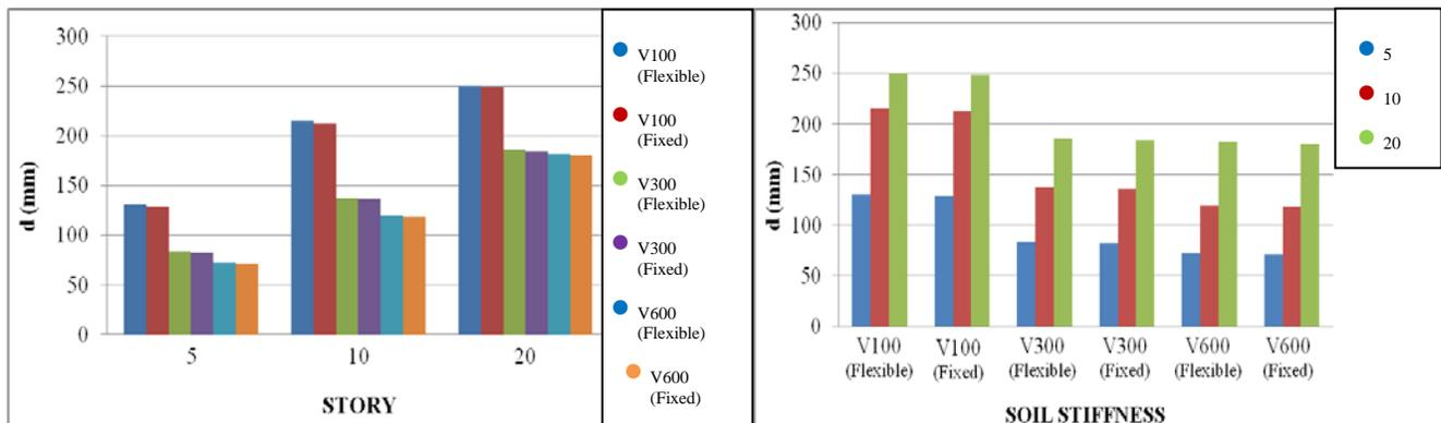
Fig. 4 – Lateral Deflection (Y direction) of different structures on different support conditions
