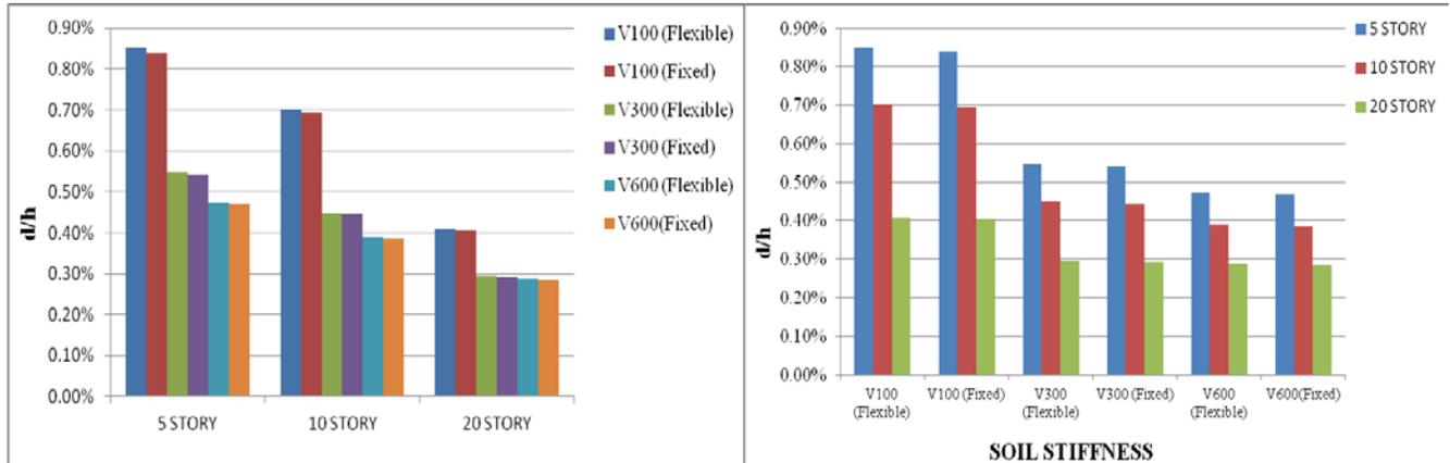
Fig. 7 – Drift ratio (X direction) of different structures on different support conditions
