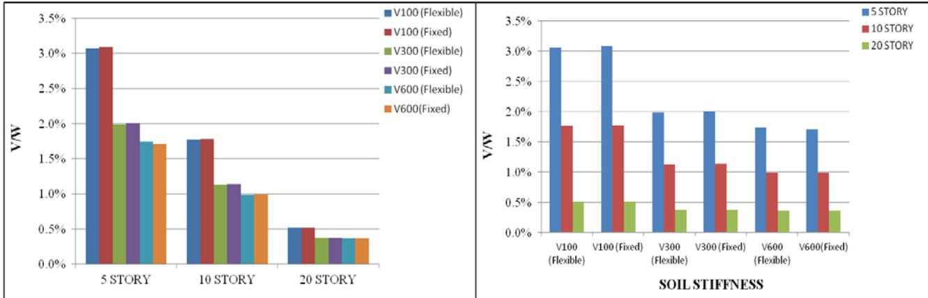
Fig. 9 – Percent (%) Base Shear (X direction) of different structures on different support conditions
