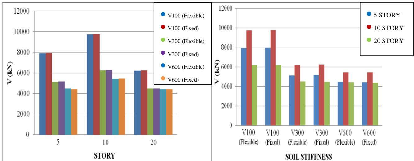
Fig. 5 – Base Shear (X direction) of different structures on different support conditions
