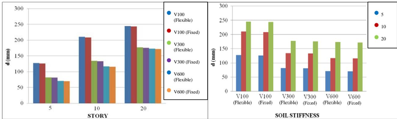
Fig. 3 – Lateral Deflection (X direction) of different structures on different support conditions
