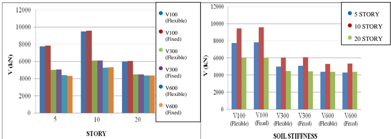
Fig. 6 – Base Shear (Y direction) of different structures on different support conditions
