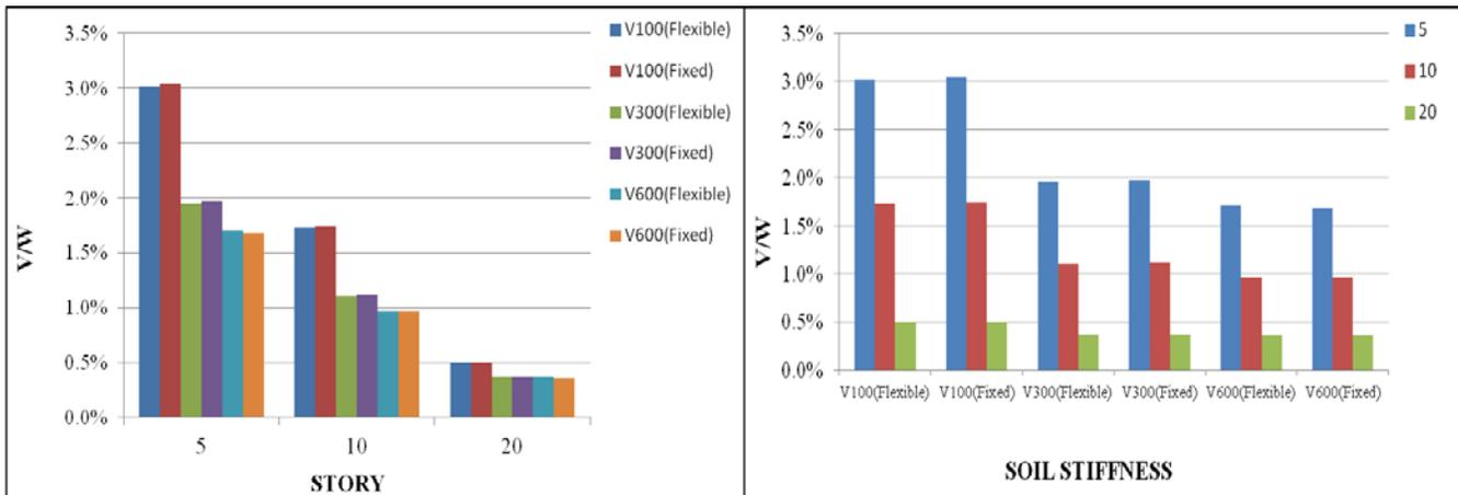
Fig. 10 – Percent (%) Base Shear (Y direction) of different structures on different support conditions
