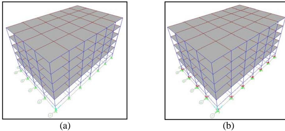
Fig. 1 – SAP2000 [9] model of Structure A, (a) Rigid base (pinned) (b) Flexible-base
