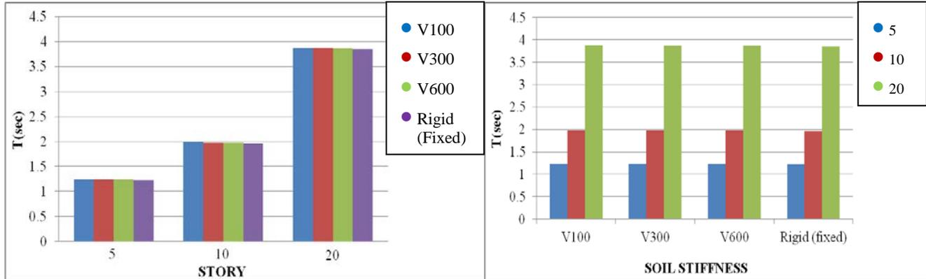
Fig. 2 – Natural Time Period (First Mode) of different structures on different support conditions
