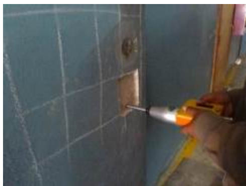
Photo A.3- Schmidt hammer test
